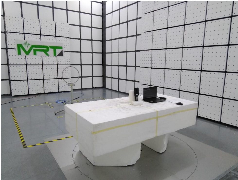
Description: Radiated Emission Test Setup for 30MHz~1GHz
