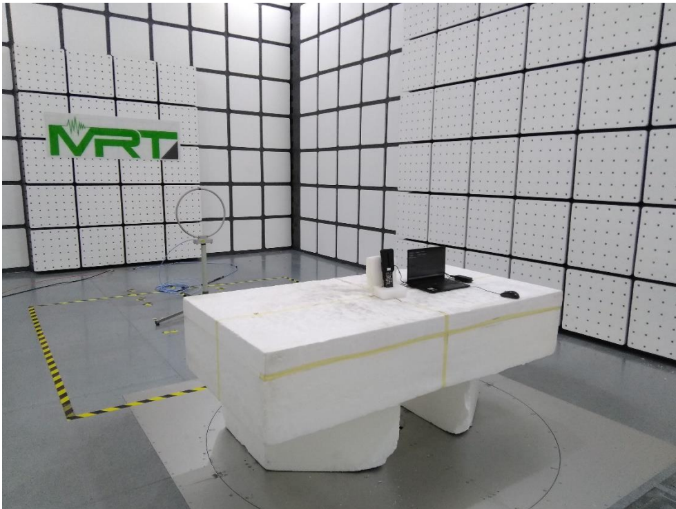
Description: Radiated Emission Test Setup for 30MHz~1GHz
