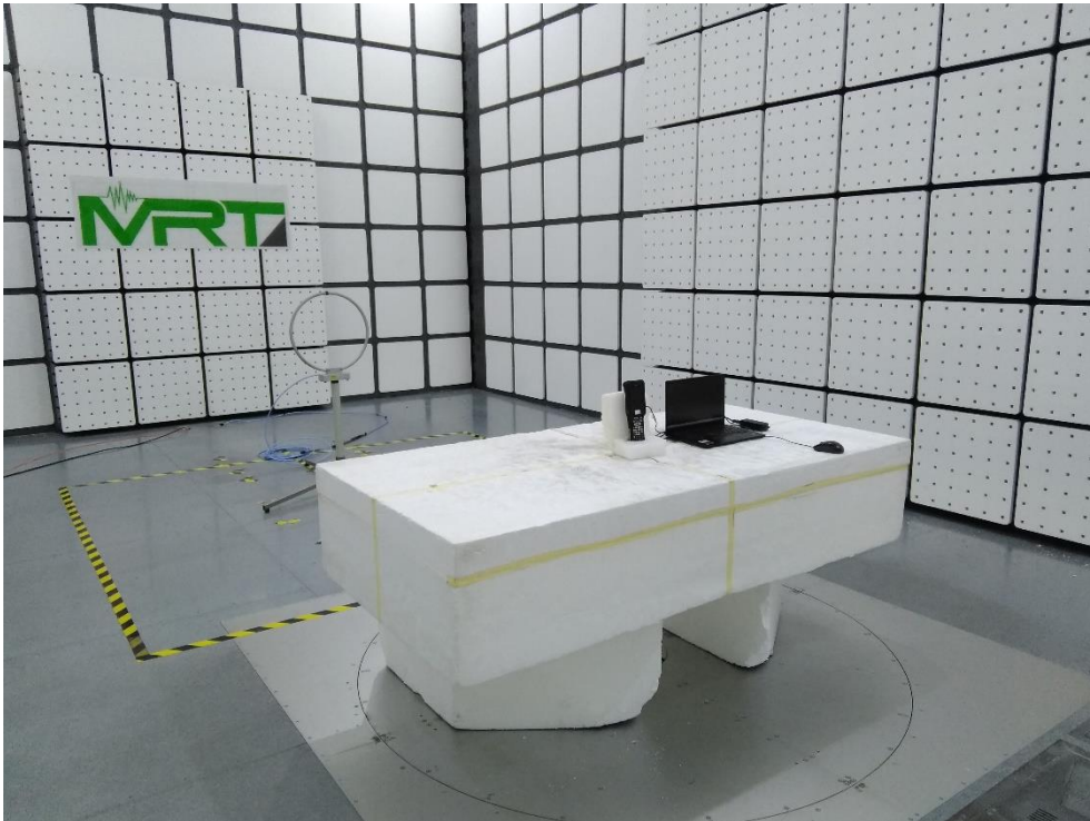
Description: Radiated Emission Test Setup for 30MHz~1GHz
