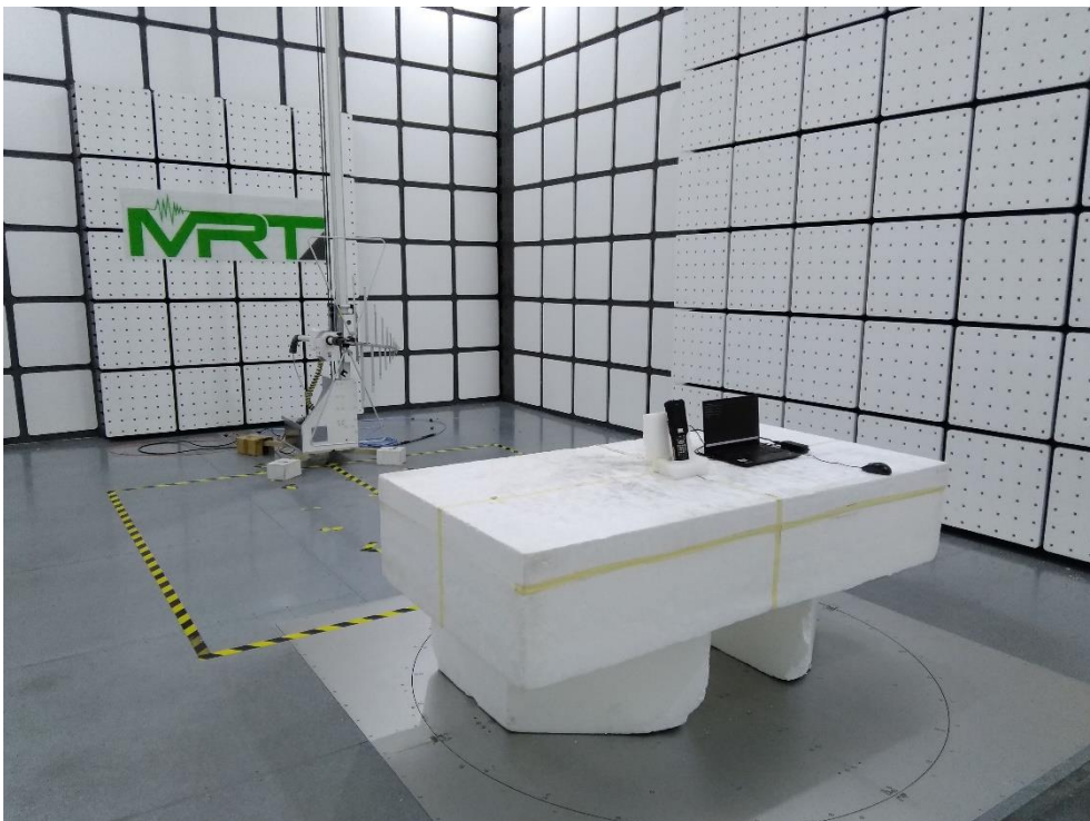
Description: Radiated Emission Test Setup for 30MHz~1GHz
