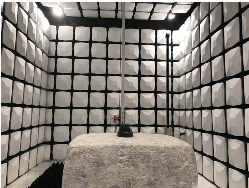
Description: Radiated Emission Test Setup for 1~18GHz
