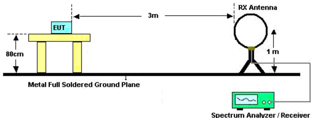
For radiated emissions from 30MHz to 1GHz
