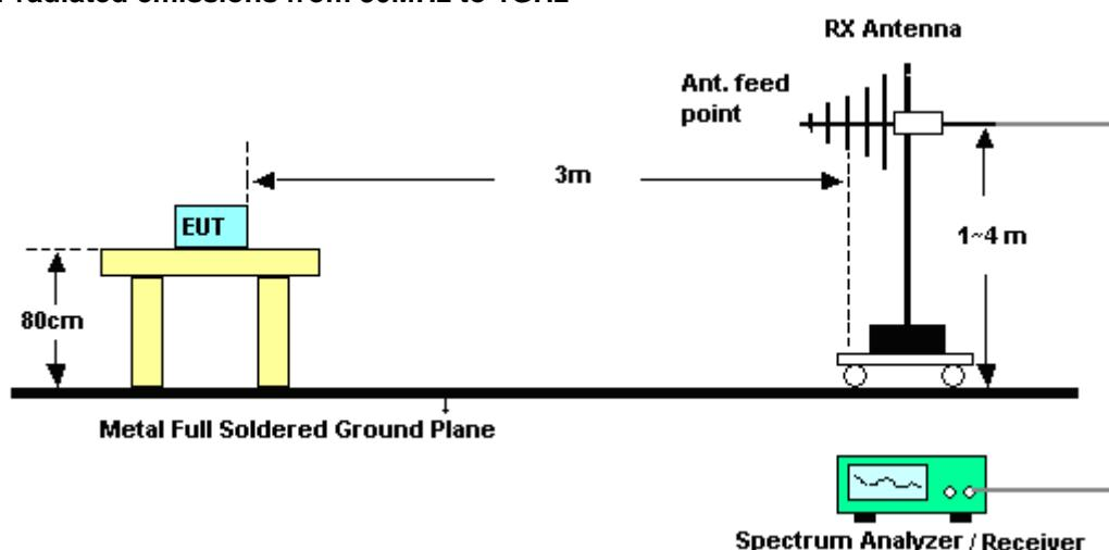
**For radiated emissions above 1GHz**
