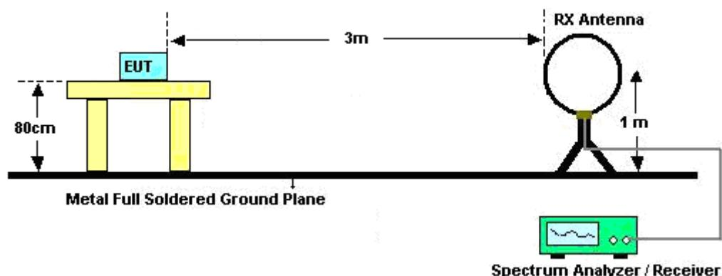
For radiated emissions from 30MHz to 1GHz
