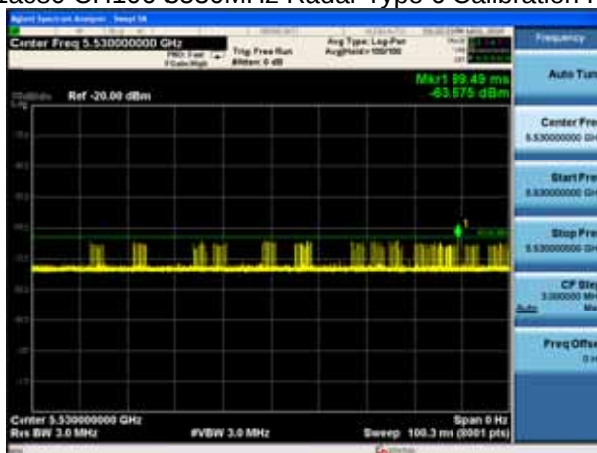
11ac80 CH106 5530MHz Radar Type 6 Calibration Plot
