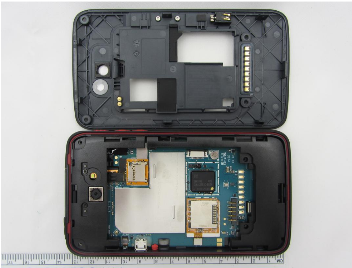
Back Side, Rear Panel Removed, Device w/ NFC (8 MP Camera & Flash, Docking Contacts)
