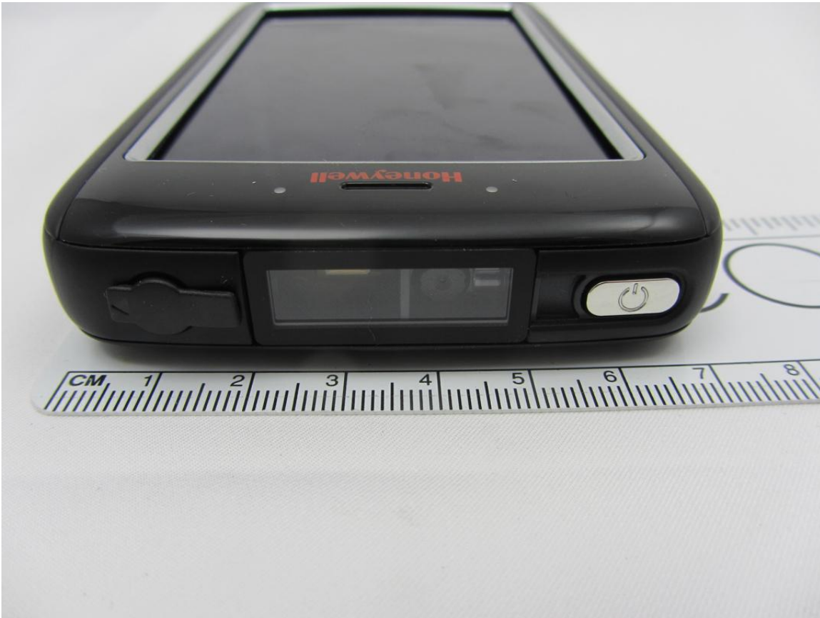
Top Side (Headphone Jack, 2D Imager, On/Off Button)
