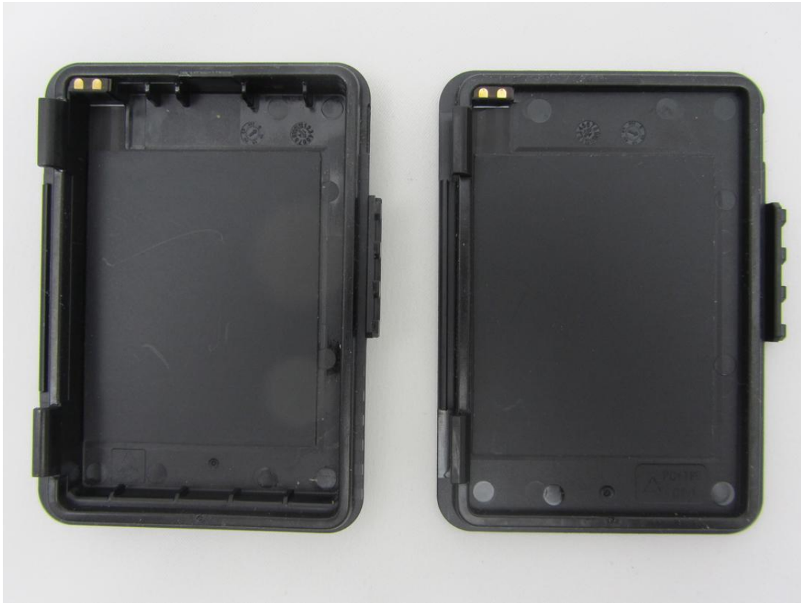
NFC Antenna (Extended Battery Door on Left, Standard Battery Door on Right)
