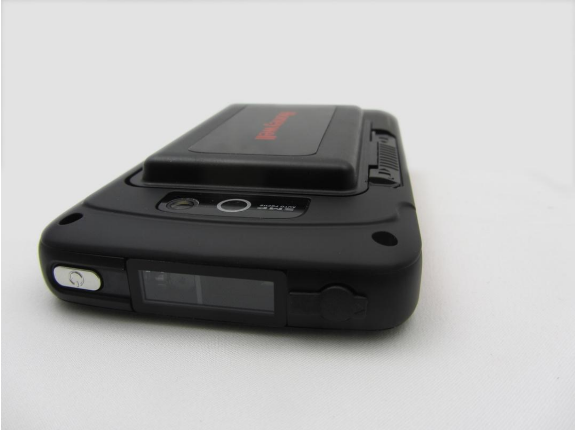
Top Side (On/Off Button, 2D Imager, Headset Jack, Extended Battery Cover)
