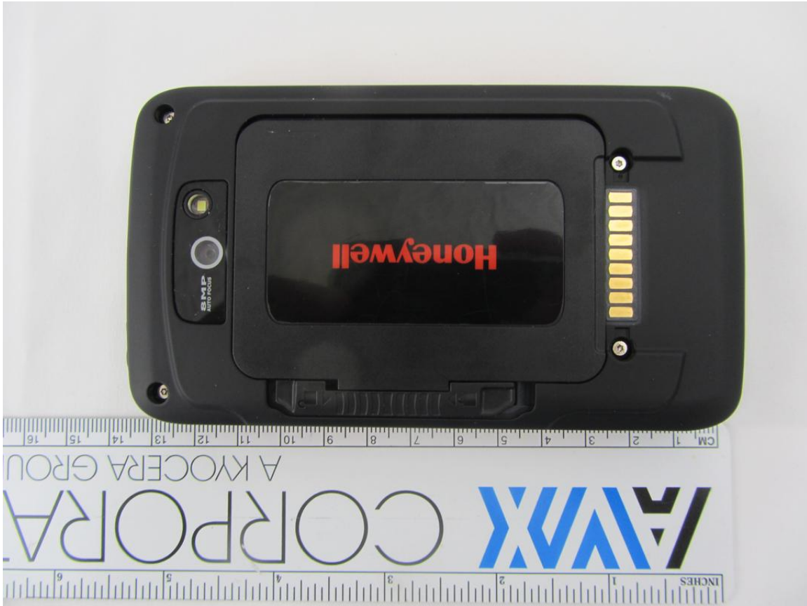
Back Side (8 MP Camera & Flash, Docking Contacts, Standard Battery Cover)
