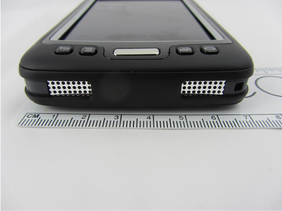
Bottom Side (Speaker, Lanyard Attachment)
