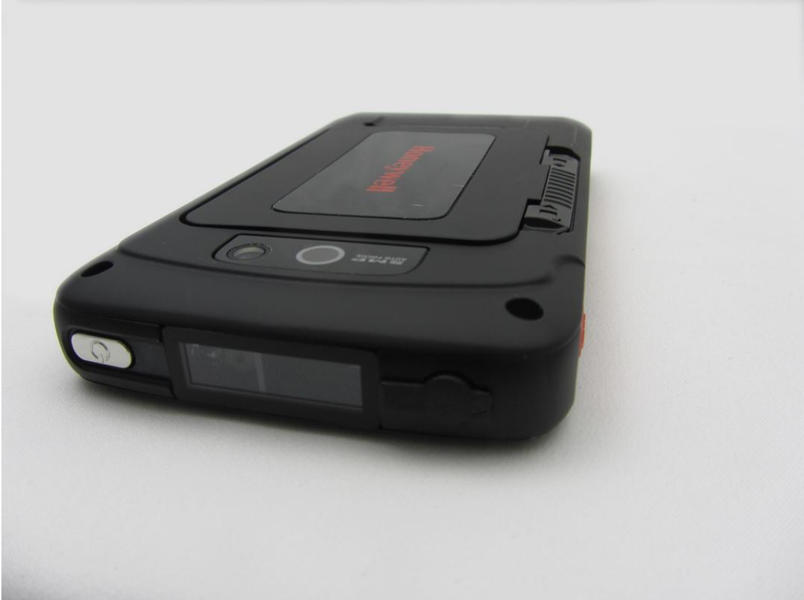
Top Side (On/Off Button, 2D Imager, Headset Jack, Standard Battery Cover)
