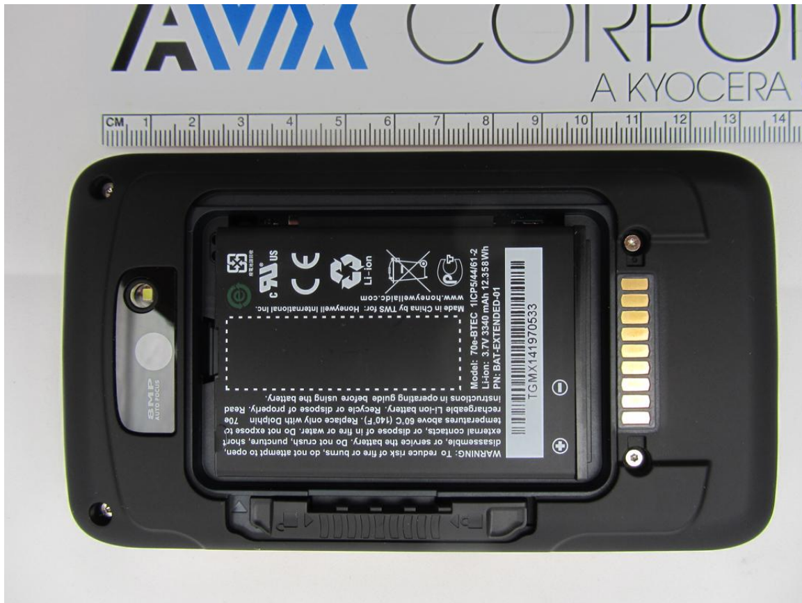
Back Side (8 MP Camera & Flash, Docking Contacts, Extended Battery Shown)
