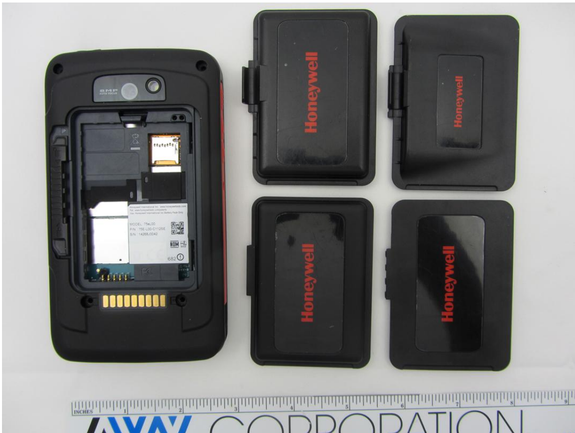
Back Side (8 MP Camera & Flash, Docking Contacts, Battery Removed, 4 Battery Cover Options)
