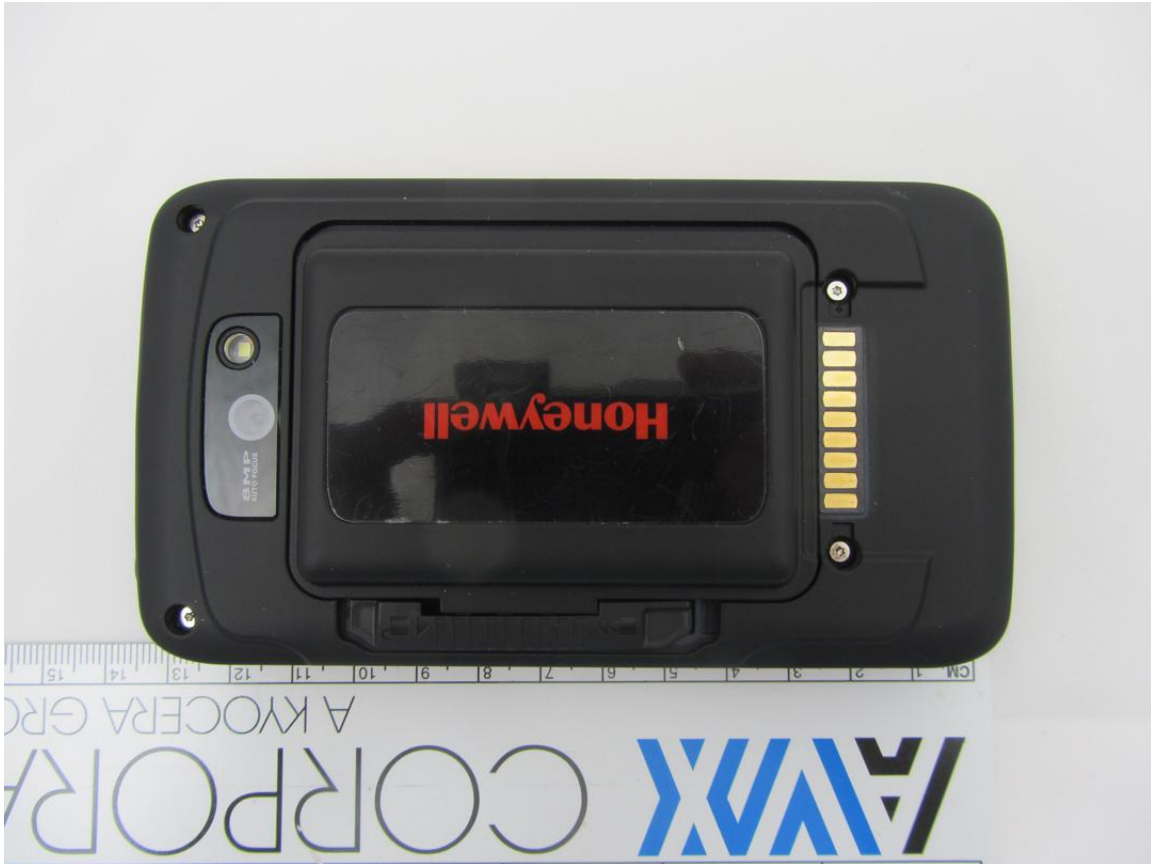
Back Side (8 MP Camera & Flash, Docking Contacts, Extended Battery Cover)
