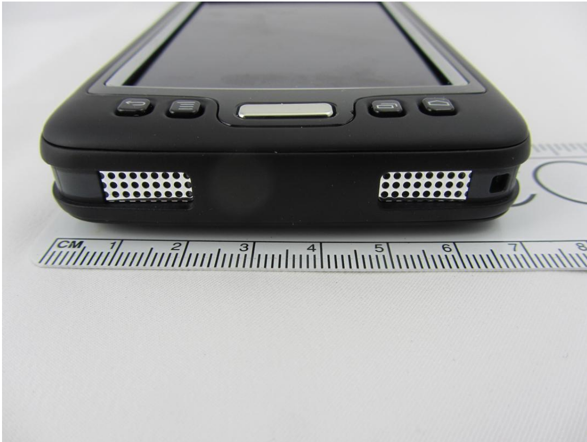
Bottom Side (Speaker, Lanyard Attachment)
