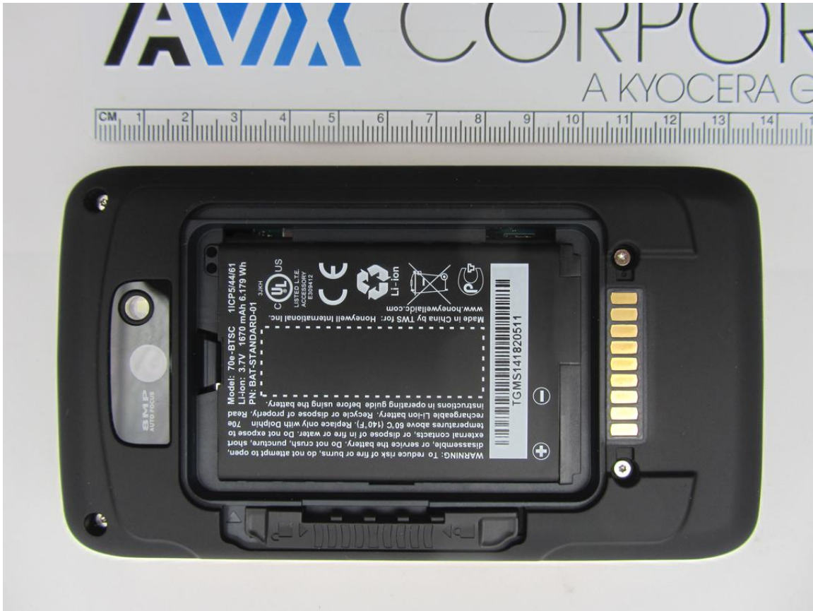
Back Side (8 MP Camera & Flash, Docking Contacts, Standard Battery Shown)
