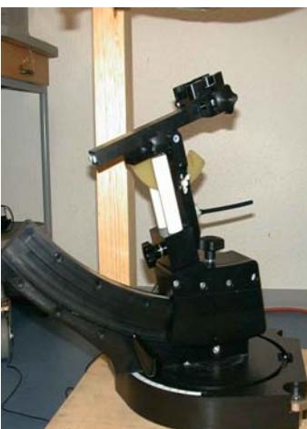
Larger DUT's (e.g. notebooks) cannot be tested using this device holder. Instead a support of bigger polystyrene cubes and thin polystyrene plates is used to position the DUT in all relevant positions to find and measure spots with maximum SAR values.
