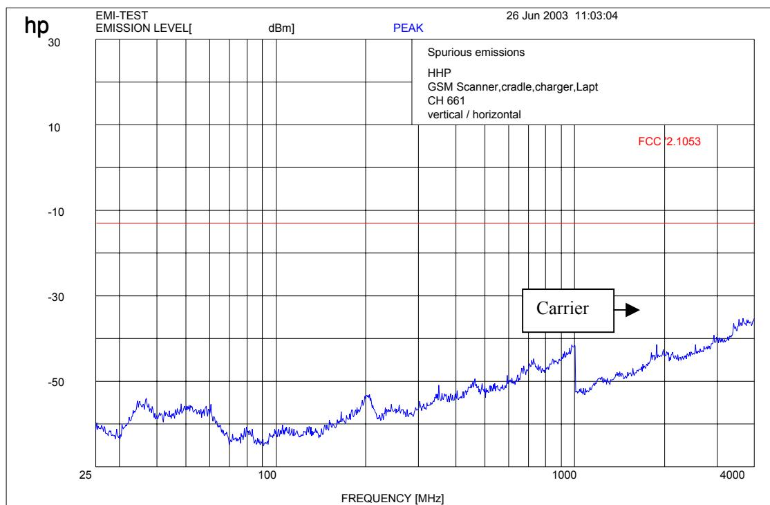
$f < 1 \text{ GHz}$  : RBW/VBW: 100 kHz $f \geq 1 \text{ GHz}$  : RBW / VBW 1 MHz**Carrier suppressed with a rejection filter****REFERENCE NUMBER(S) OF TEST EQUIPMENT USED**
