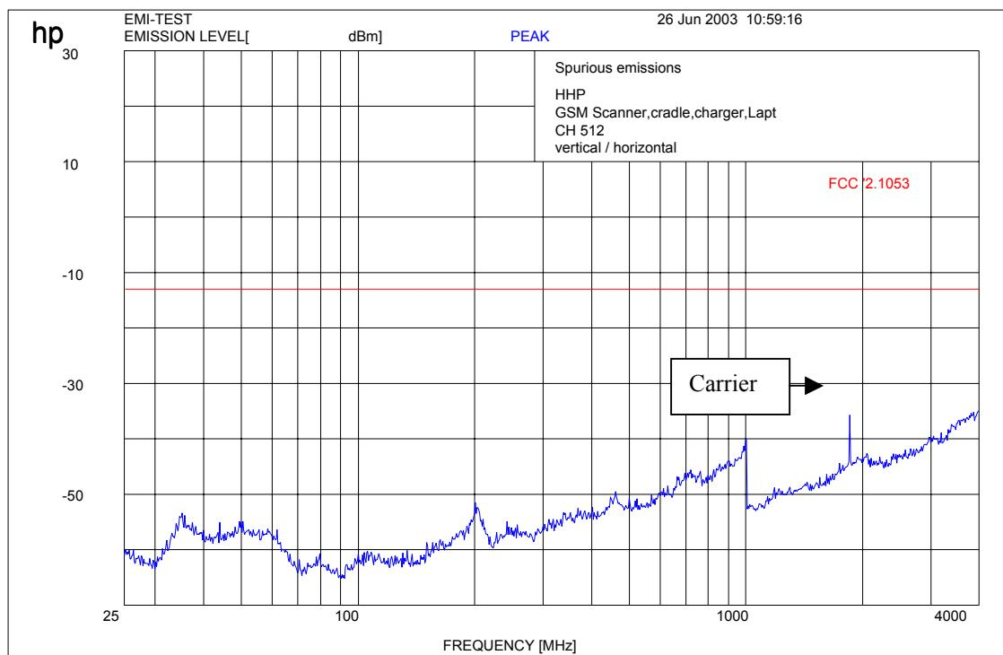
**f < 1 GHz : RBW/VBW: 100 kHz****f ≥ 1GHz : RBW / VBW 1 MHz****Carrier suppressed with a rejection filter****REFERENCE NUMBER(S) OF TEST EQUIPMENT USED****(for reference numbers see test equipment listing)****17 – 24; 64**
