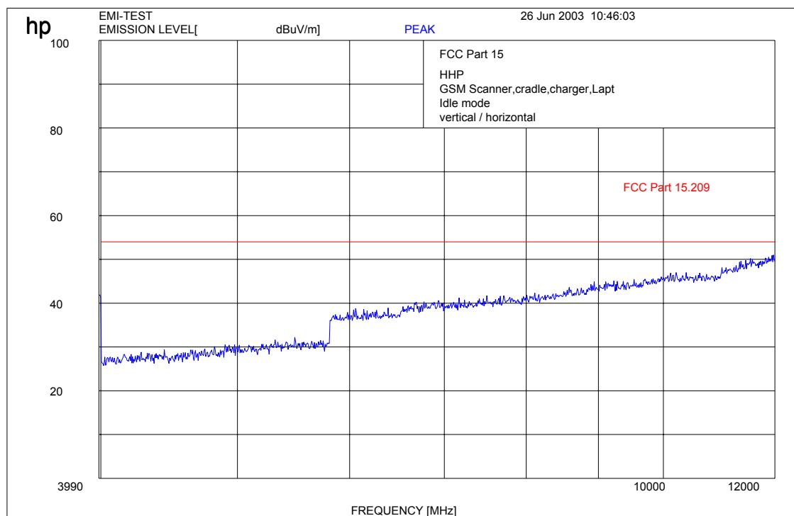
**f < 1 GHz : RBW/VBW: 100 kHz****f ≥ 1GHz : RBW/VBW 1 MHz****REFERENCE NUMBER(S) OF TEST EQUIPMENT USED****(for reference numbers see test equipment listing)****17 – 24, 64**
