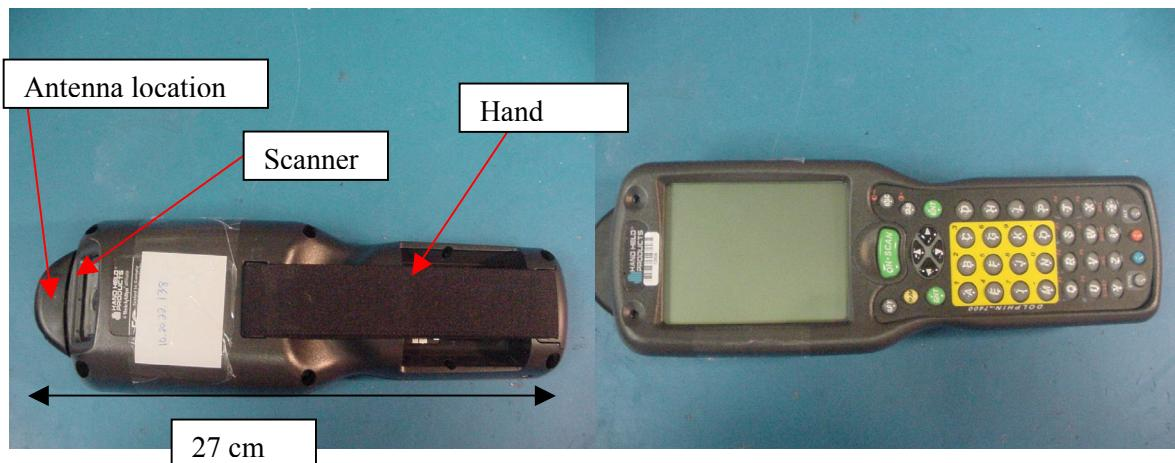
By design, the antenna operates with a separation distance of at least 2.5 cm from a person's hands, wrists, feet and ankles, and the peak conducted and peak radiated (EIRP) output power do not exceed 11mW. After data collection using the scanner/imager feature, the Dolphin 7400 is normally placed in its HomeBase terminal or cradle. During normal operation, the device and its antenna operate at more than 5 cm from a person's body.
