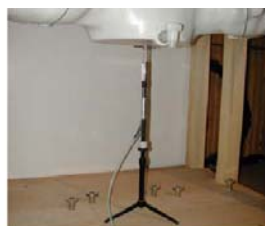
Figure 9.1 Dipole Verification Test Setup Diagram & Photo
