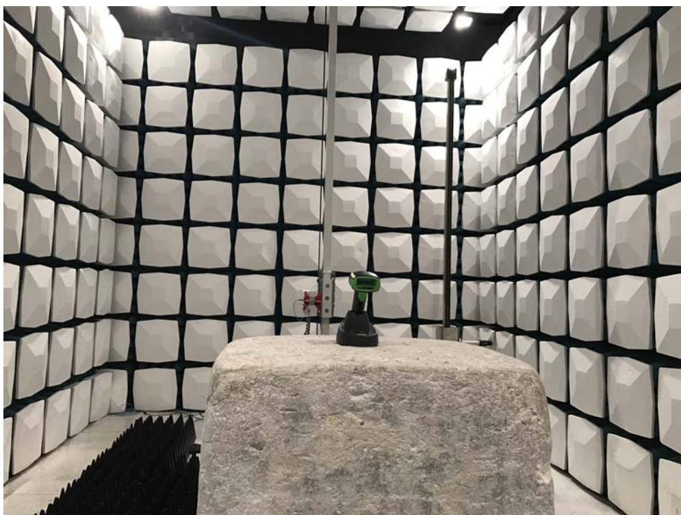
Description: Radiated Emission Test Setup for 1~18GHz
