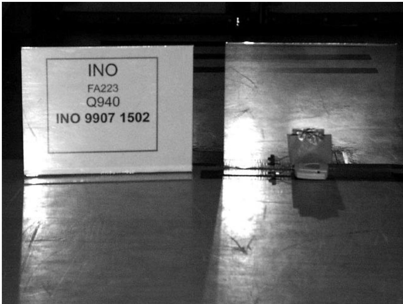
**Part 3.2 Radiated Emissions Orientation 2 Setup - Front View**
