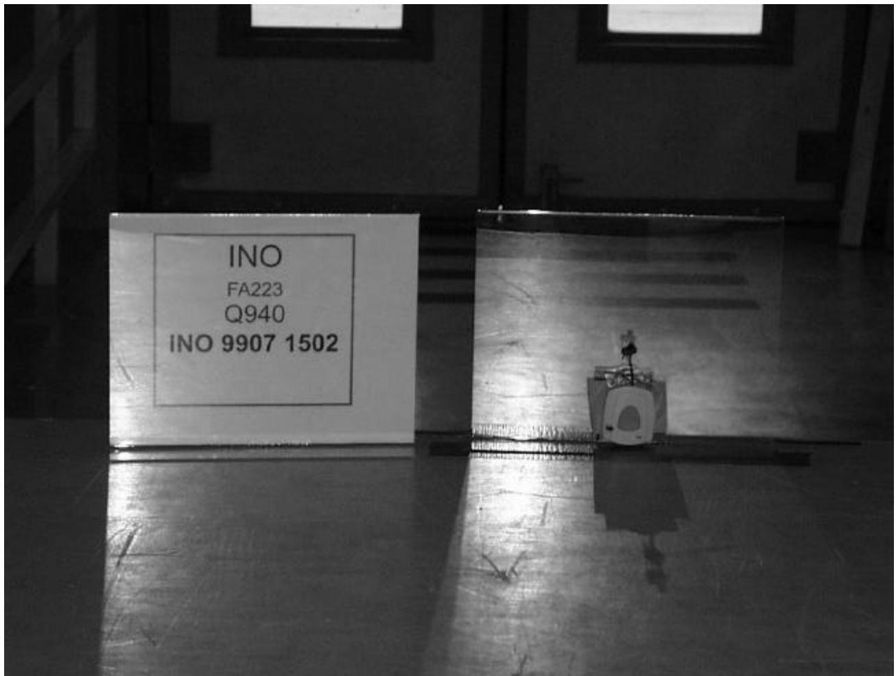
**Part 3.4 Radiated Emissions Setup, 1 to 10 GHz - Rear View**
