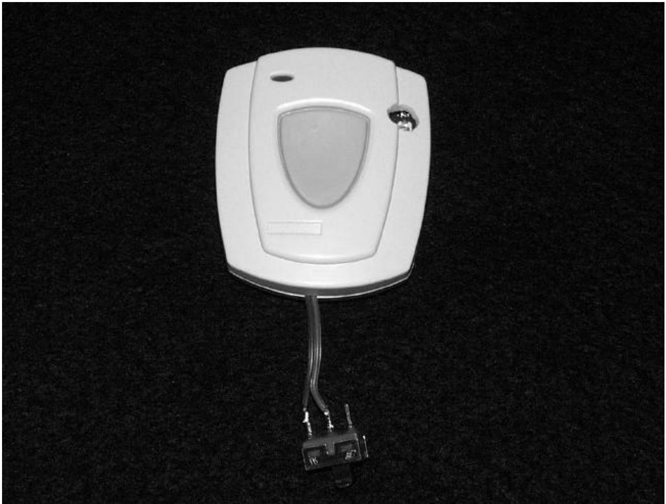
**Note:** The toggle switch is not a part of the production version of this device. It was used to enable the three frequency continuous hop sequence used during the test (fo low, mid, and high).
