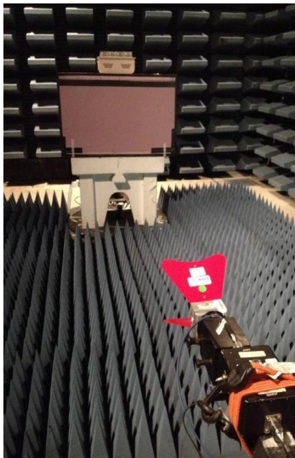
Figure 3: Radiated Emissions (Above 1GHz) Emissions Test Setup
