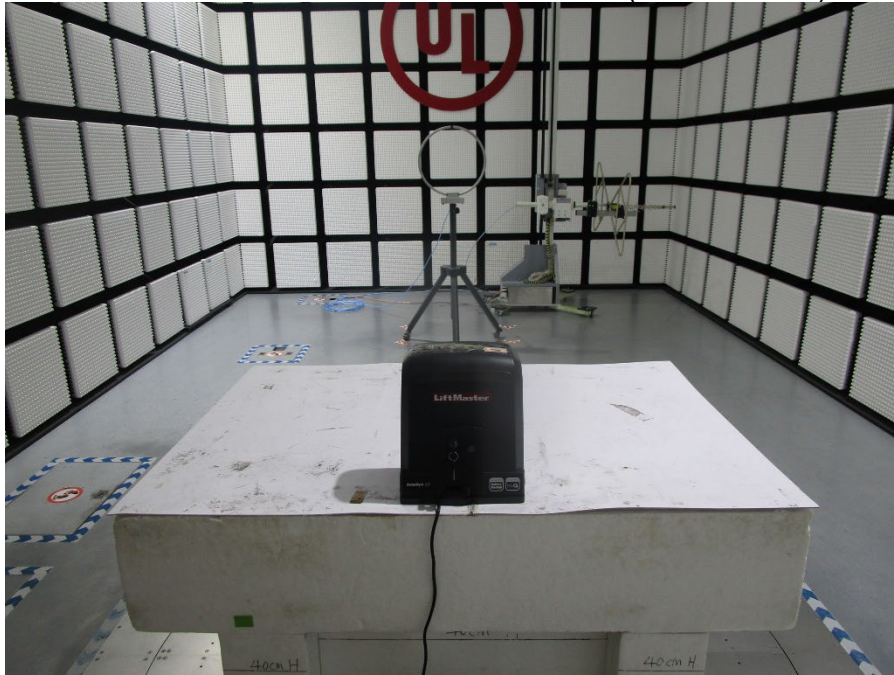
RADIATED RF MEASUREMENT SETUP (Below 30MHz)
