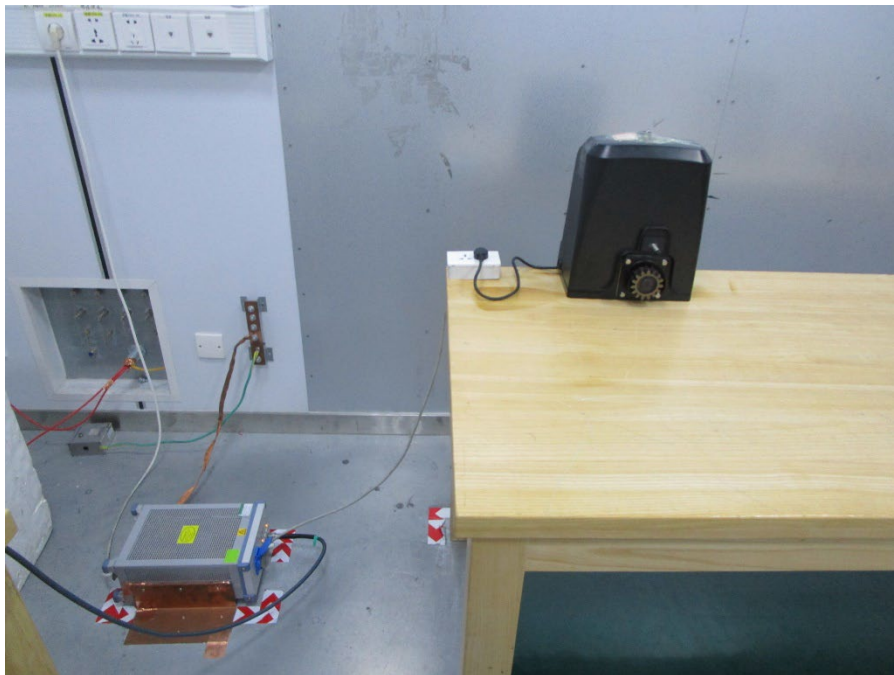
POWERLINE CONDUCTED EMISSIONS MEASUREMENT SETUP
