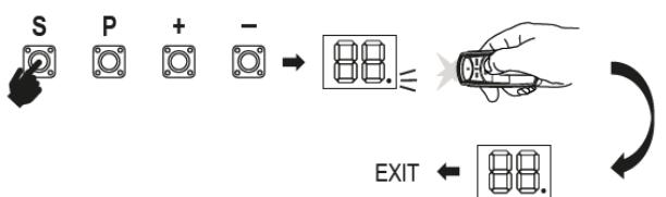
Your gate opener receiver and one of the buttons remote control are pre-programmed. If you purchase additional remote controls, the gate opener must be programmed to accept the new remote code.
