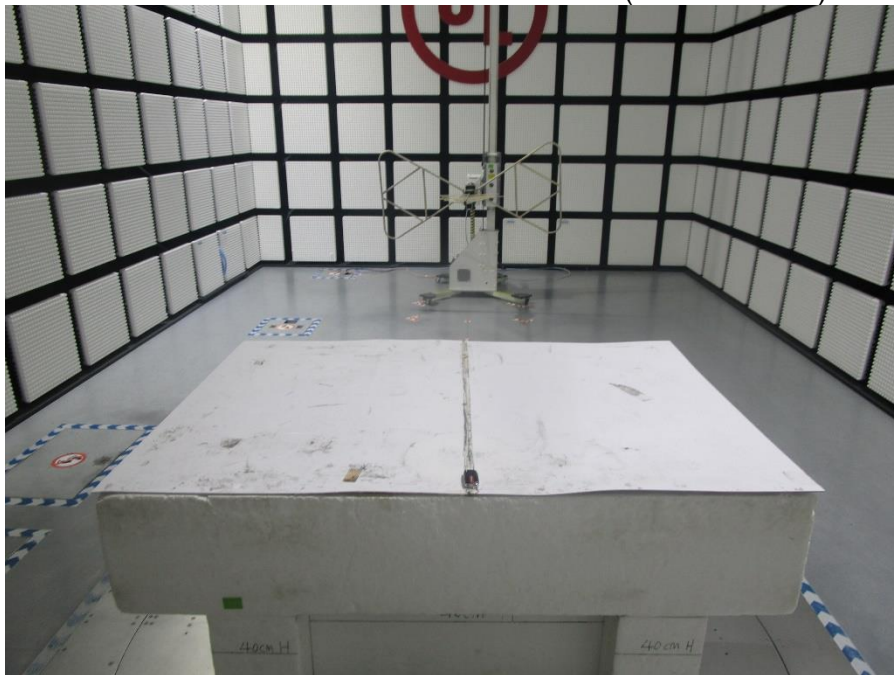
RADIATED RF MEASUREMENT SETUP (30MHz~1GHz)
