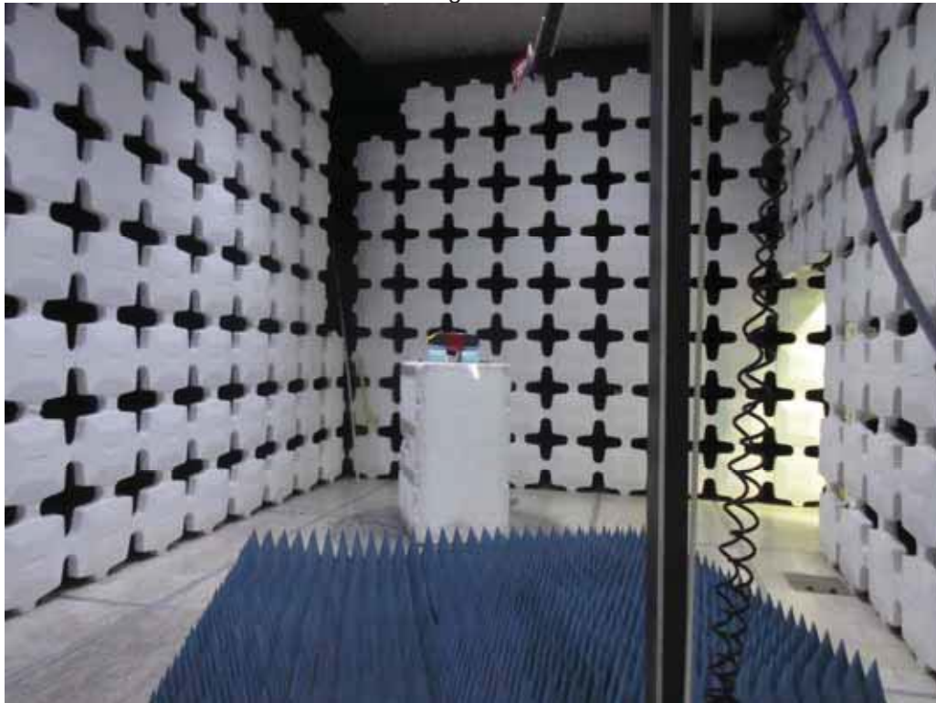
Test Setup for Radiated Emissions (Transmitter) – 1 to 10GHz, Horizontal Polarization
