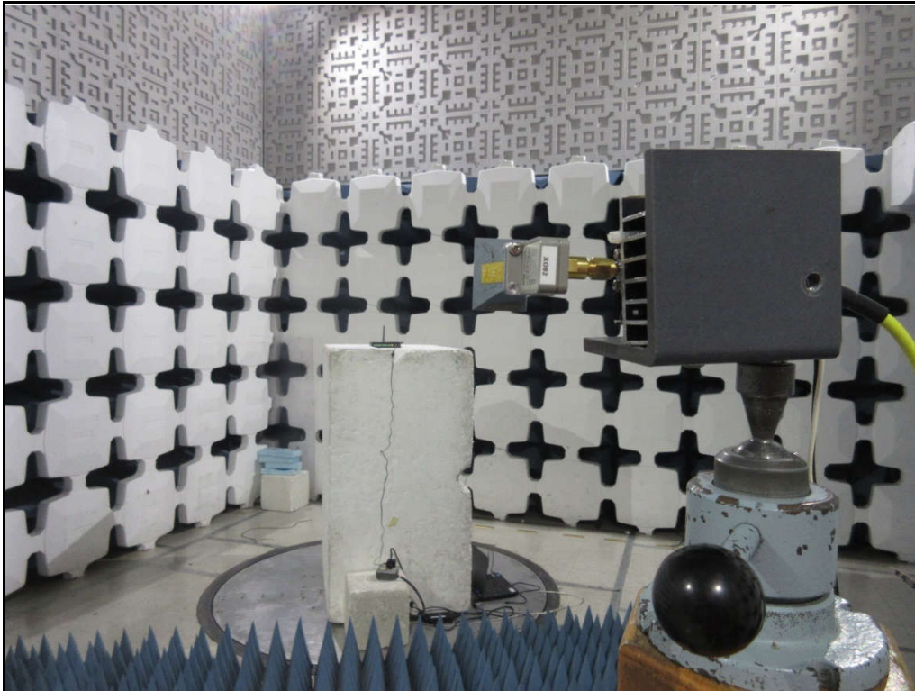
Test Setup for Spurious Radiated Emissions, 18 – 25GHz – Antenna Polarization Horizontal
