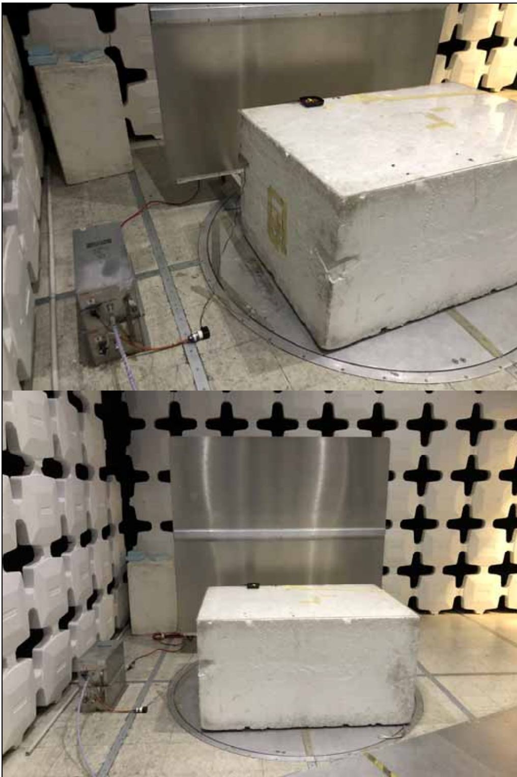
Test Setup for RF Conducted Emissions (AC Mains)
