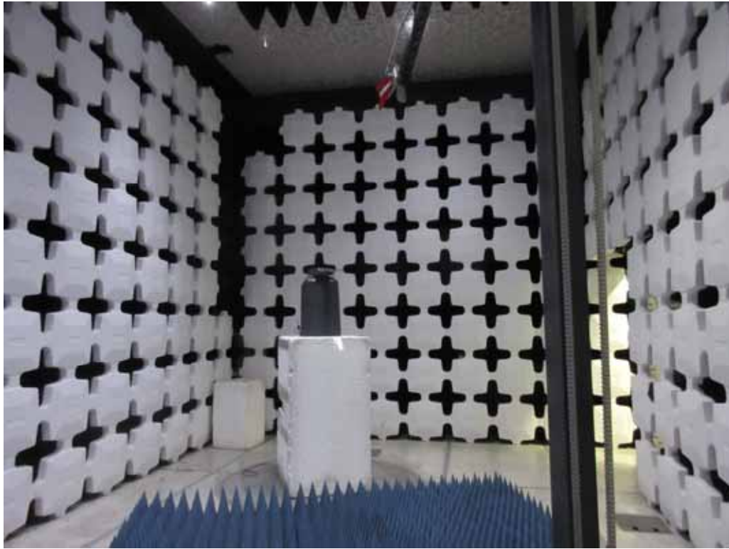
Test Setup for Spurious Emissions – 1 to 10GHz, Horizontal Polarization
