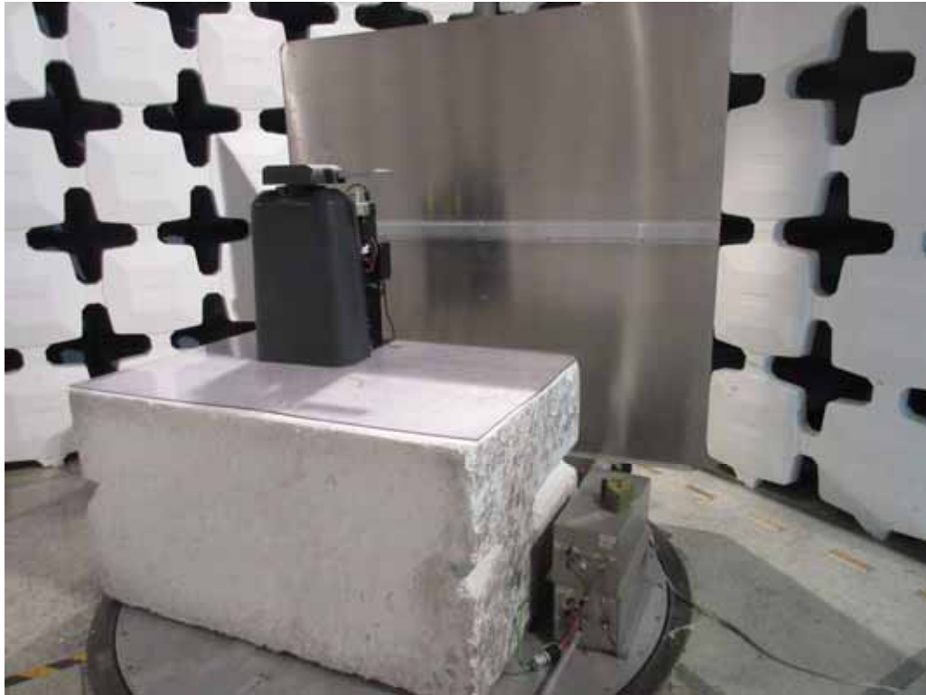
Test Setup for Conducted Emissions
