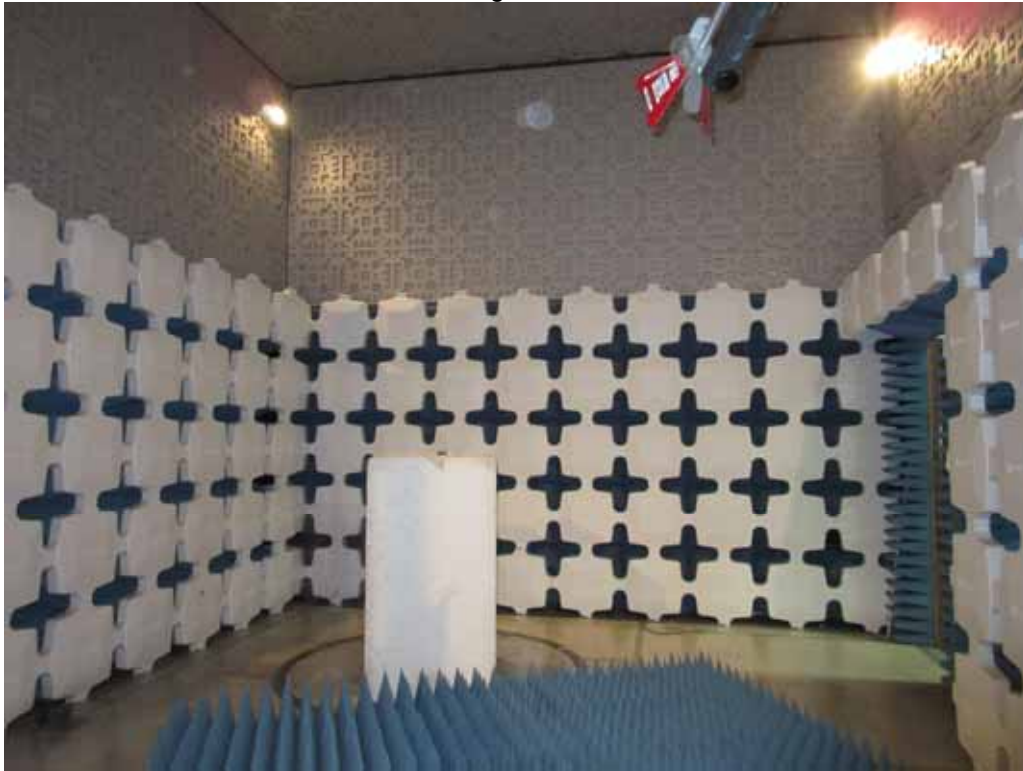
Test Setup for Radiated Emissions, 1-4.5GHz – Horizontal Polarization
