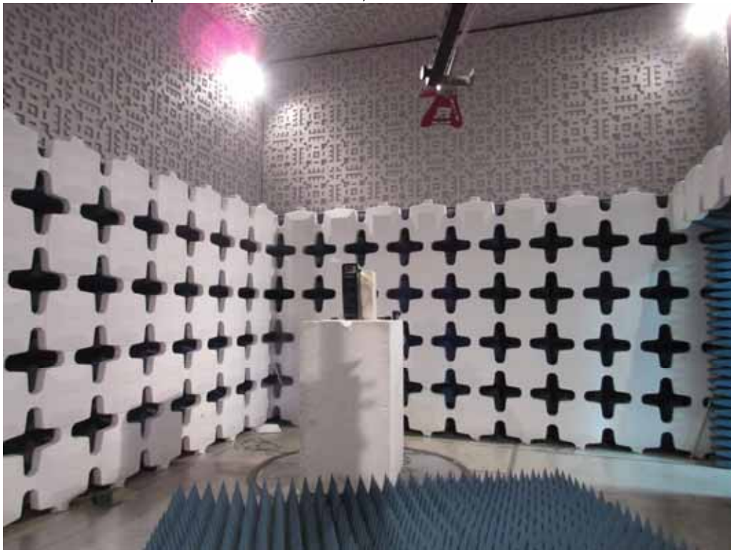
Test Setup for Radiated Emissions, 1 - 10GHz – Vertical Polarization
