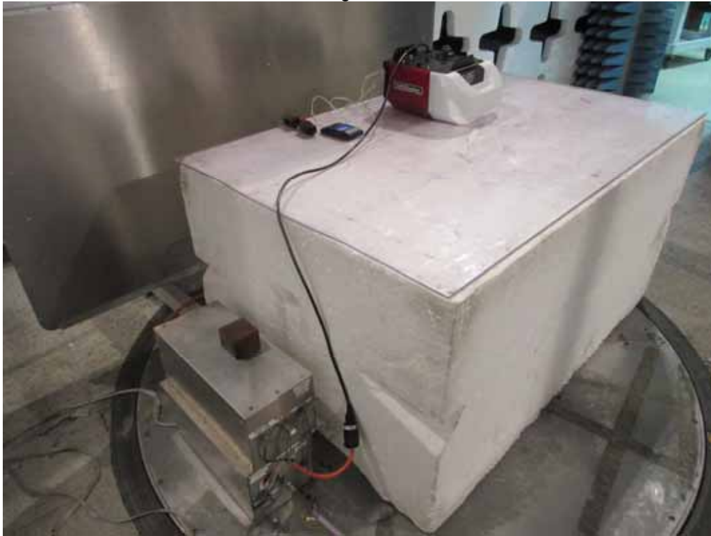
Test Setup for Conducted Emissions
