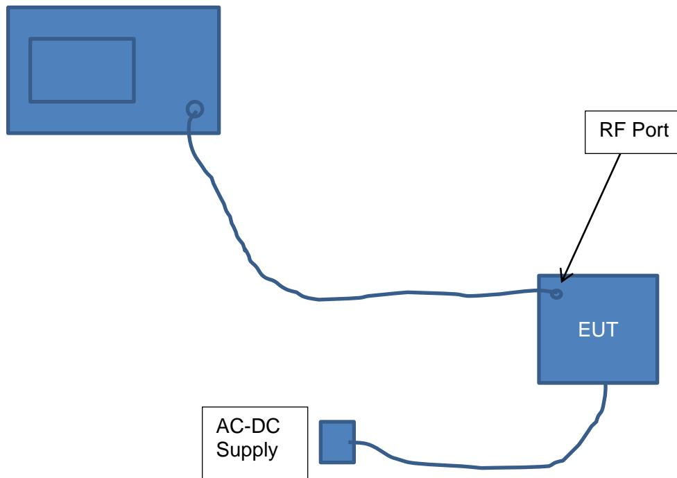
**RADIATED RF MEASUREMENT SETUP**
