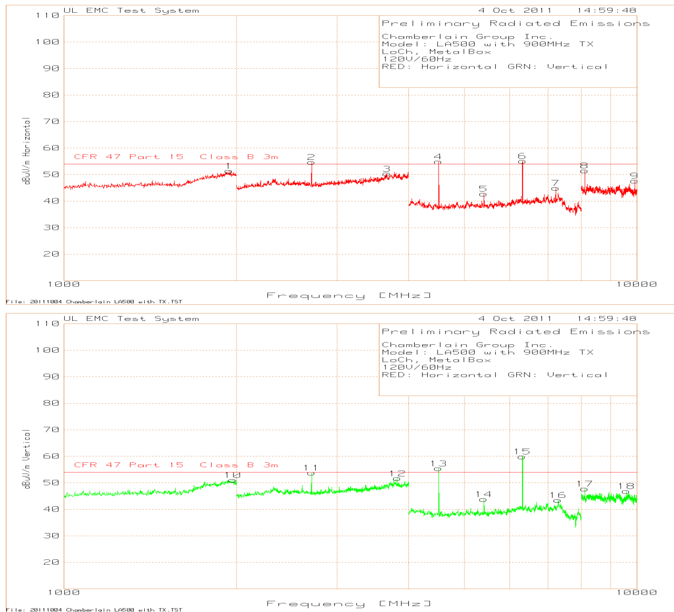
Figure 18 Radiated Spurious Emissions above 1GHz, Low Channel (Metal Enclosure)
