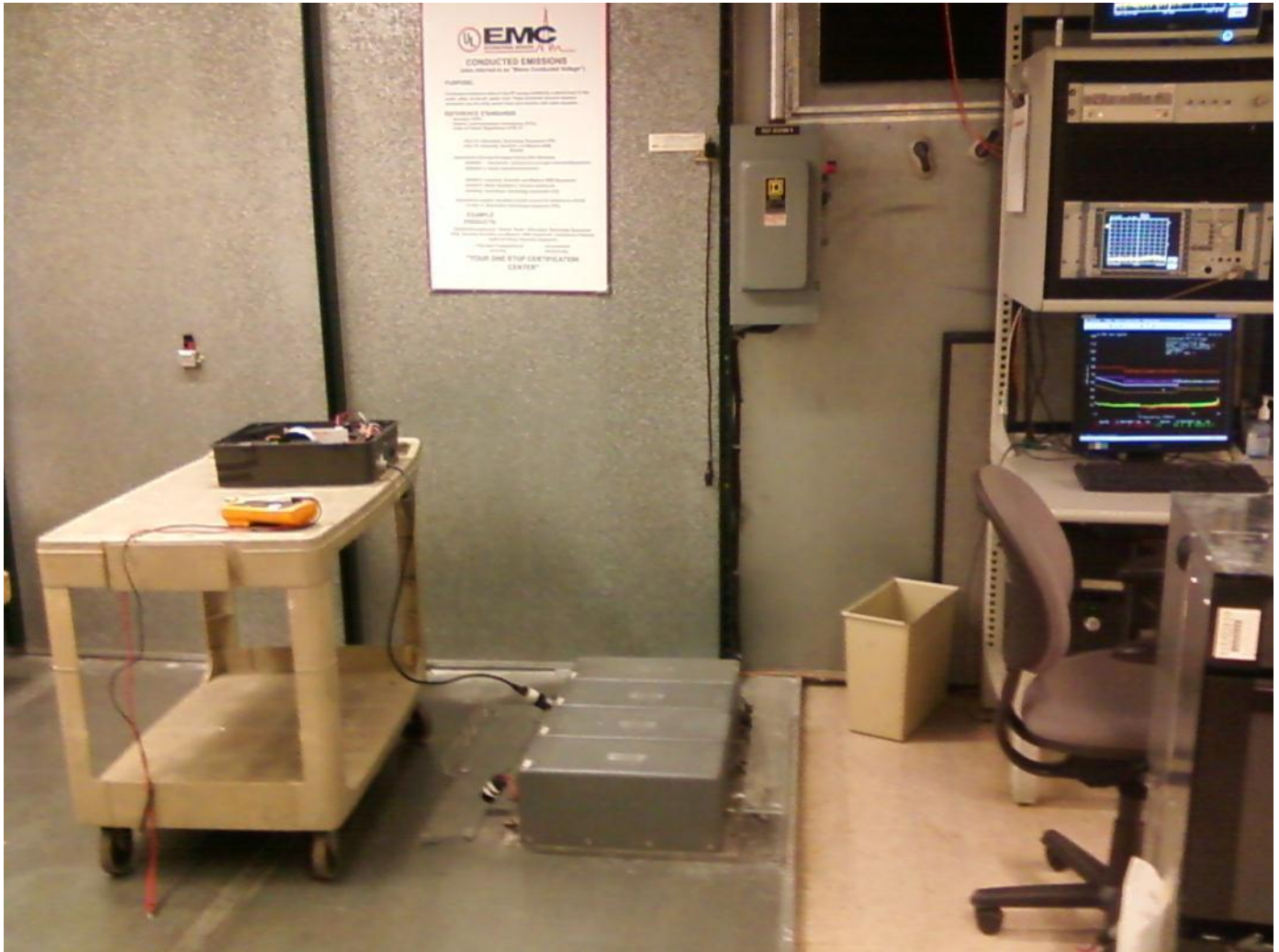
Figure 1 Test Setup for Conducted Emissions
