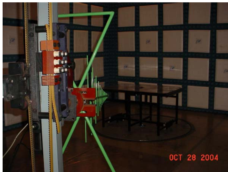
Test Setup for Radiated Emissions Vertical Polarity
