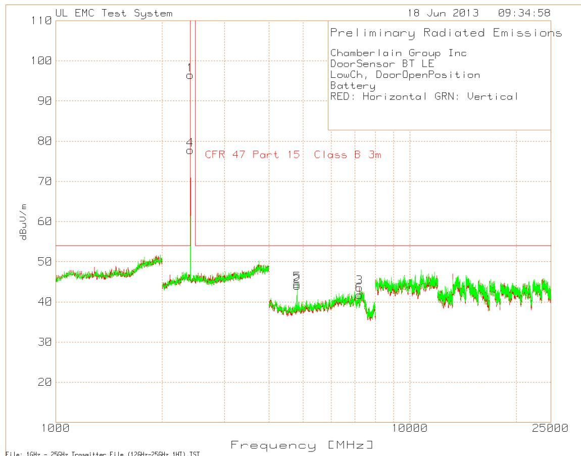
Based on peak pre-scan data all emissions are attenuated at least 6dB under the limit. Further measurements were considered not required.
