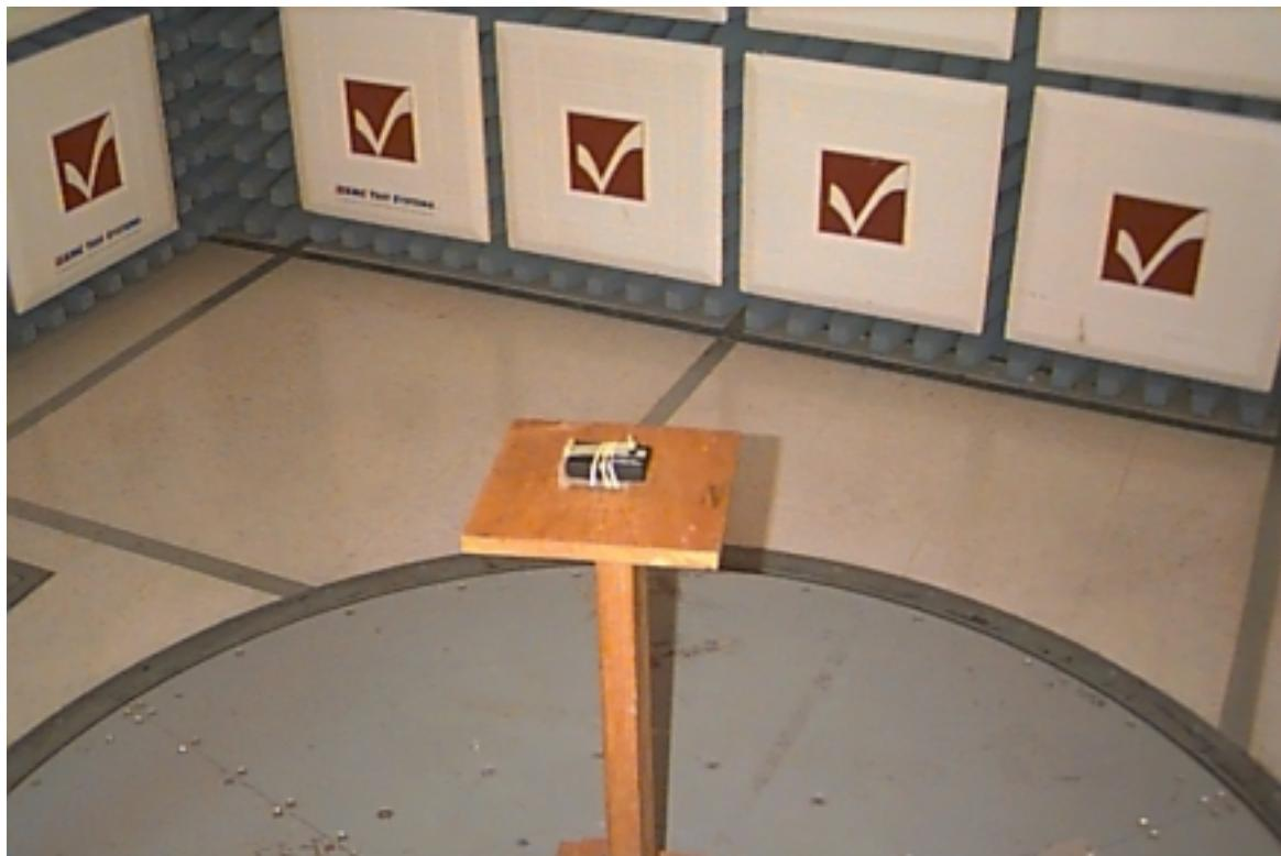
View of the Remote Control transmitter during the Radiated Emissions tests. This view shows the orientation of the product where the maximum signal levels were present in the horizontal polarity. In order to cause the remote transmitter to run continuously, a small plexiglass fixture can be seen which pushes a plunger down on the appropriate button to activate transmission.
