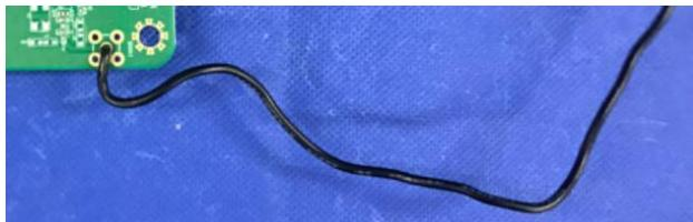
Antenna transmission frequency: 315MHz, 390MHz
