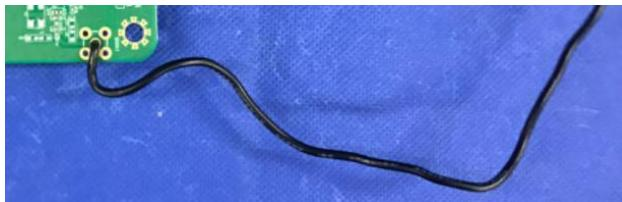
Antenna transmission frequency: 315MHz
