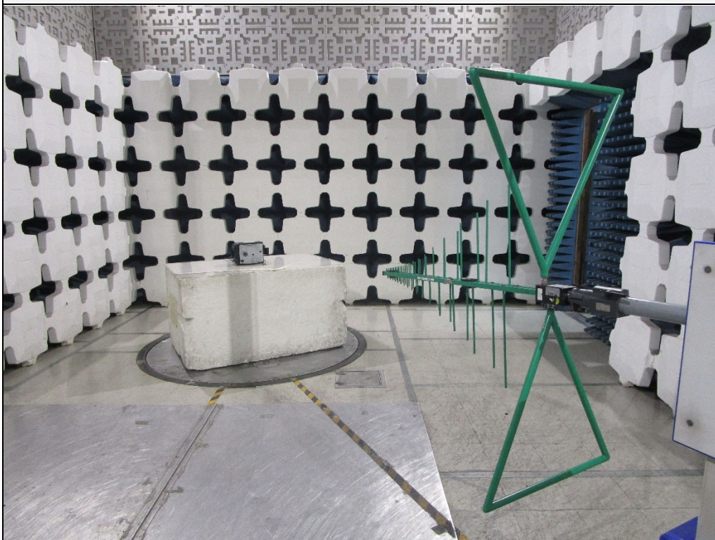
Test Setup for Spurious Emissions: 30MHz to 1GHz, Vertical Polarization
