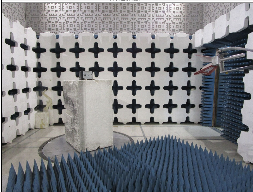
Test Setup for Spurious Radiated Emissions, 1 – 18MHz – Antenna Polarization Vertical
