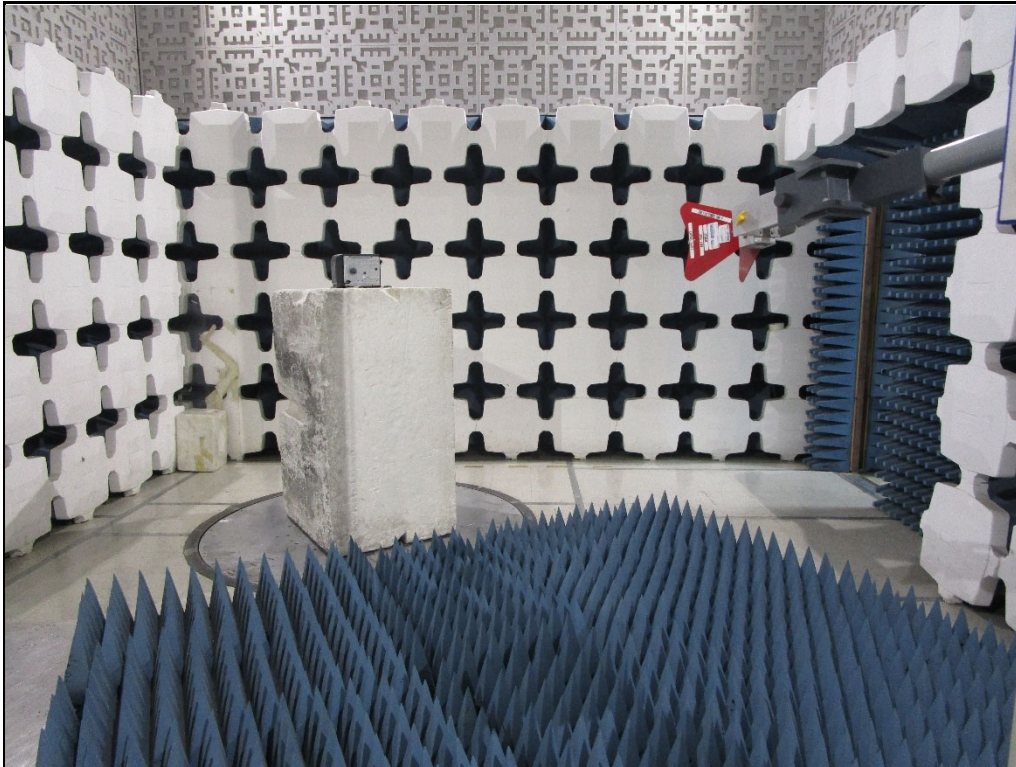
Test Setup for Spurious Radiated Emissions, 1 – 18MHz – Antenna Polarization Horizontal
