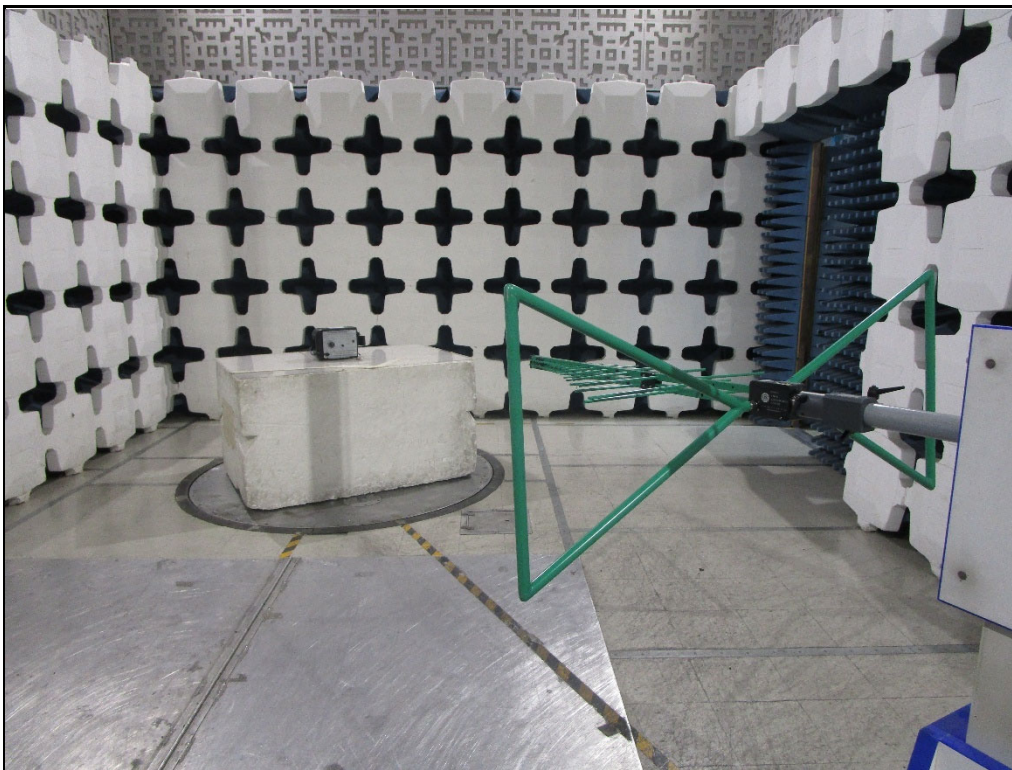
Test Setup for Spurious Radiated Emissions, 30MHz – 1GHz – Antenna Polarization Horizontal
