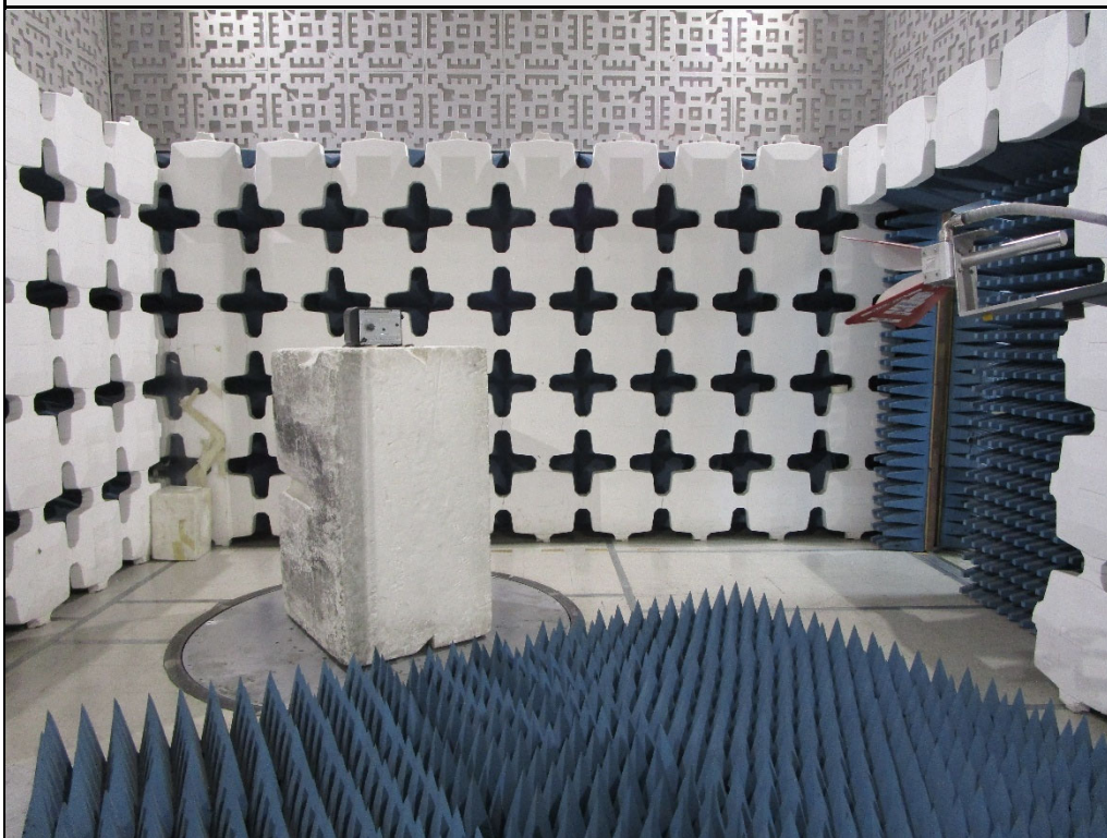
Test Setup for Spurious Radiated Emissions, 1 – 18MHz – Antenna Polarization Vertical
