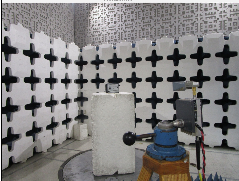
Test Setup for Spurious Radiated Emissions, 18 – 26MHz – Antenna Polarization Vertical
