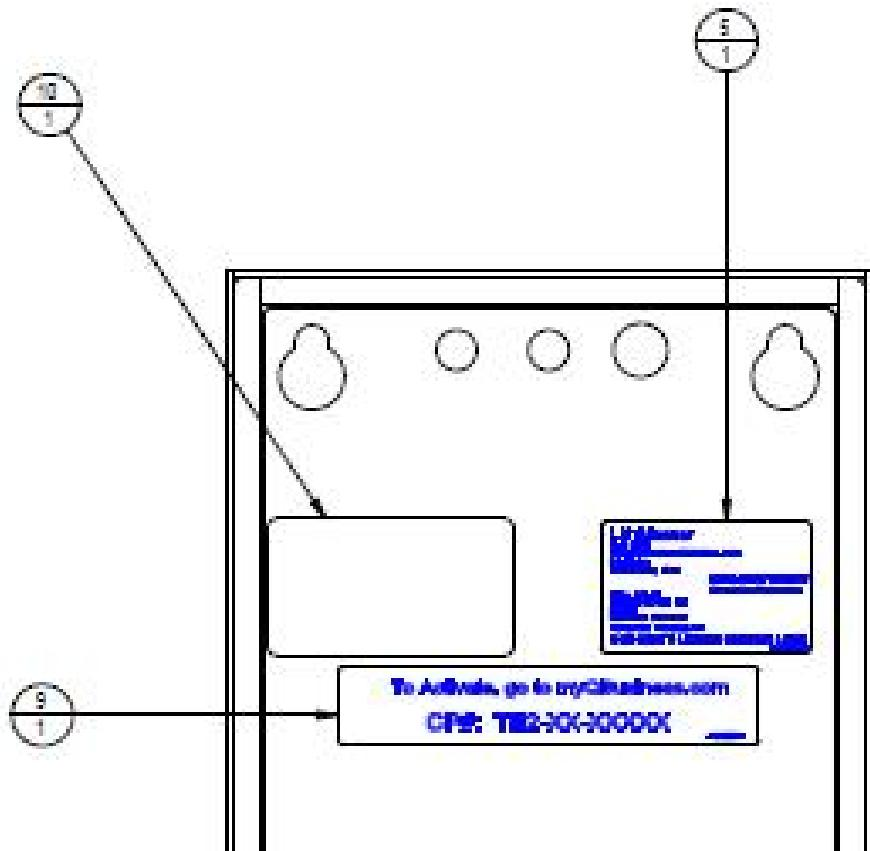
The FCC/ISED label is the blank label in the upper left corner of the enclosure cover.
