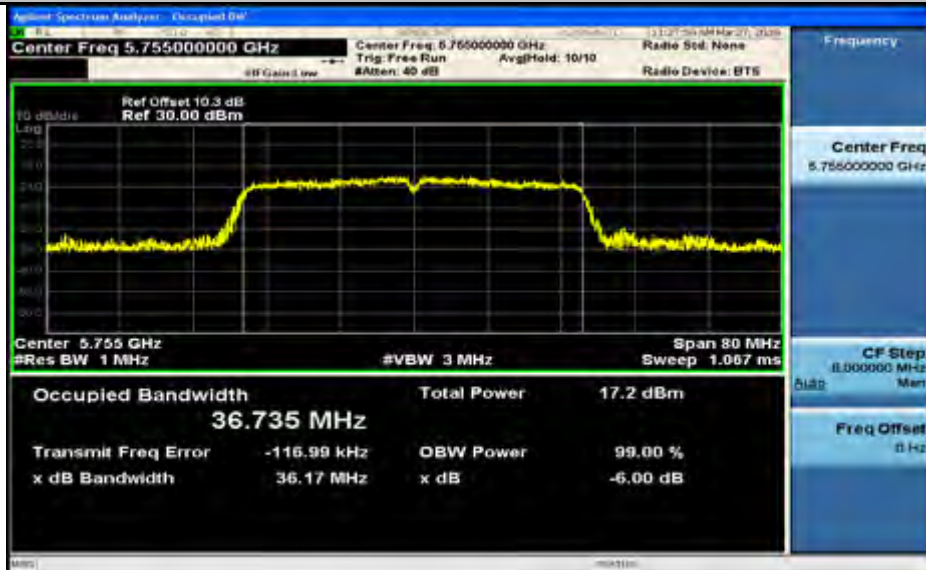
Occupied Bandwidth Measurement_11AC40_5795_Ant1
