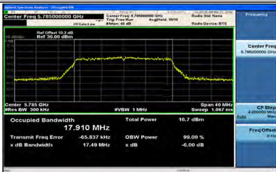
Occupied Bandwidth Measurement_11AC20_5825_Ant1
