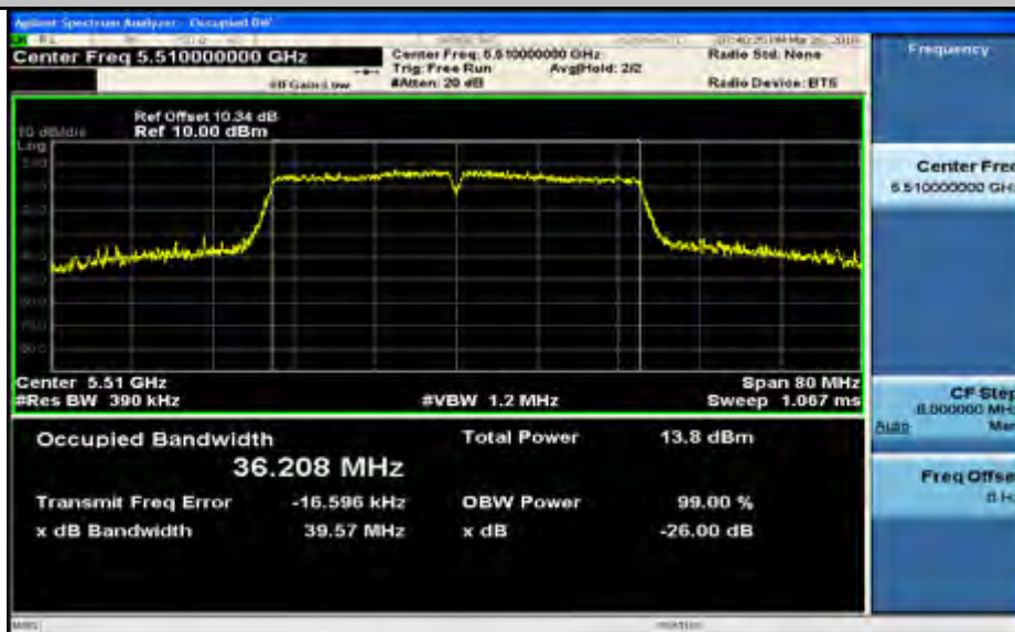
Emission Bandwidth Measurement_11N40_5590_Ant1
