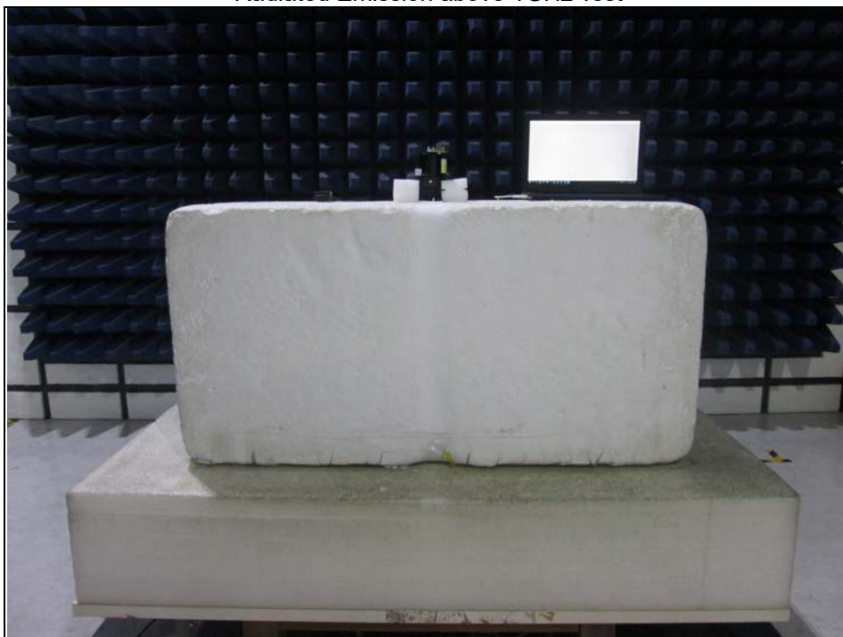
Radiated Emission above 1GHz Test
