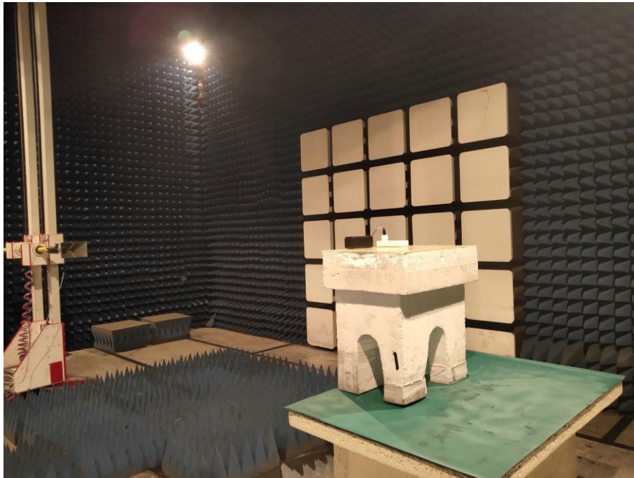
Photograph 3: Set-up for Radiated Spurious Emission, Above 1GHz
