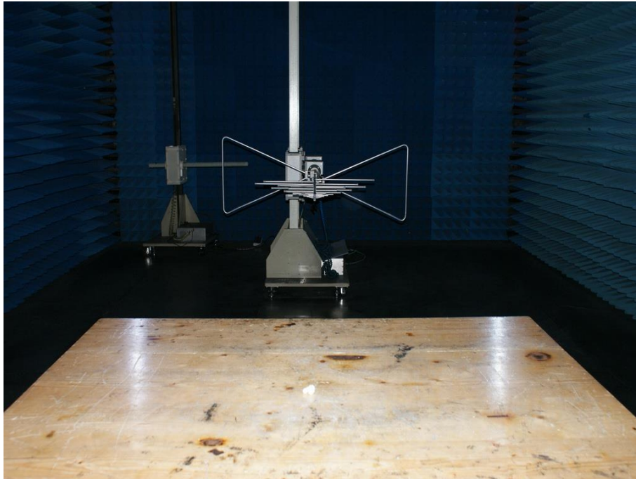
Photograph 5: Set-up for Radiated Spurious Emission, 30MHz - 1GHz
