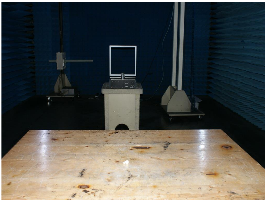
Photograph 4: Set-up for Radiated Spurious Emission, below 30MHz
