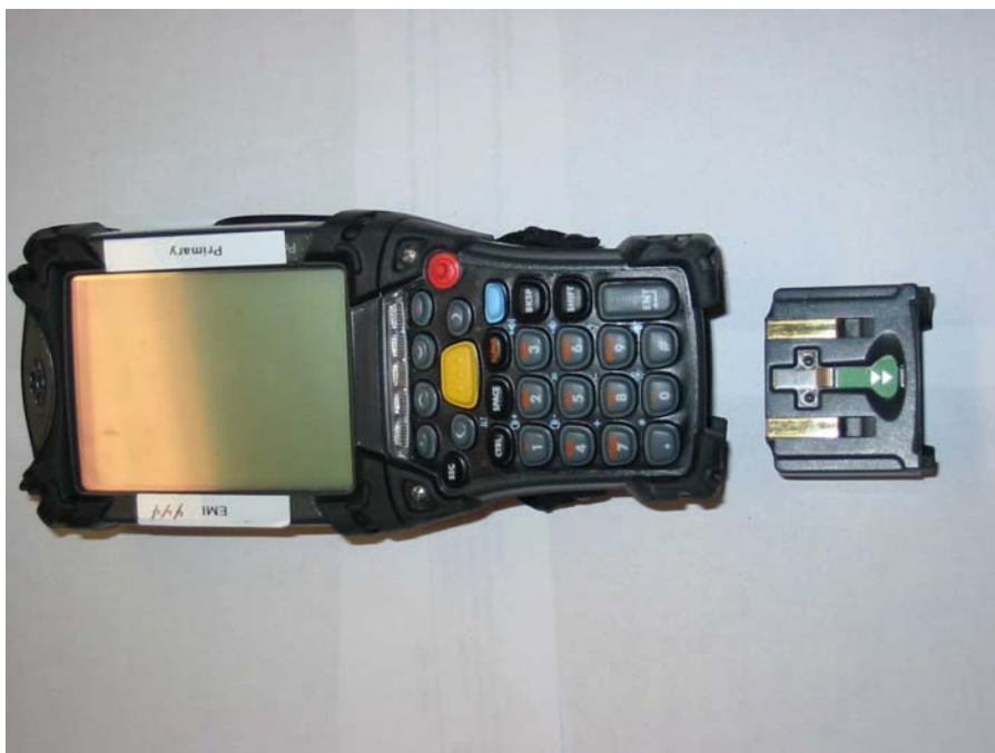
Figure 4 – MC9063 with Battery Removed
