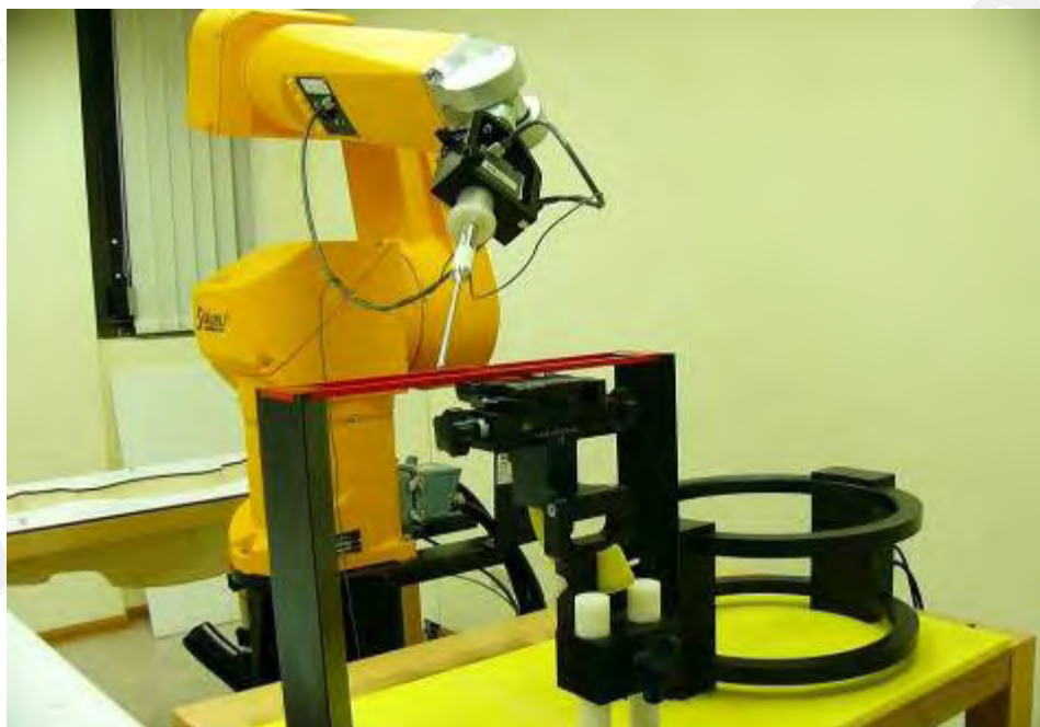
Fig.1 Photograph of the DASY 4 measurement System
