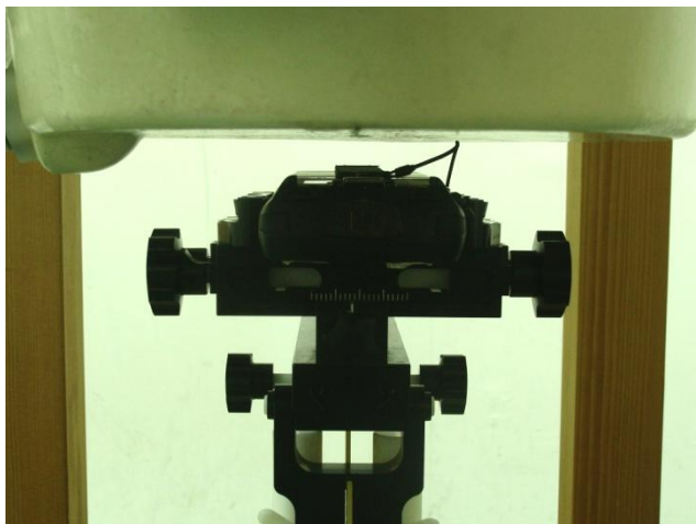
Bottom of the DUT with Battery 1 + Scanner 1 + Keypad 1 (with Phantom 1.5 cm Gap)
