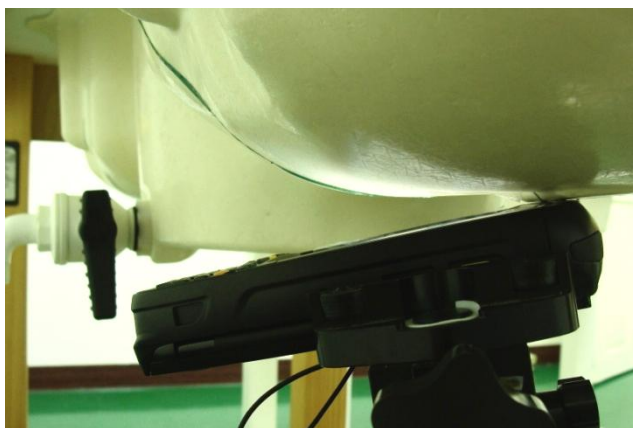
Left Tilted - DUT with Battery 1 + Scanner 1 + Keypad 3
