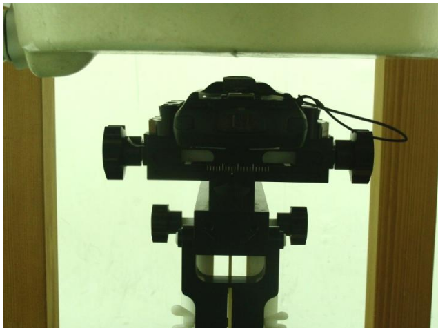
Bottom of the DUT with Battery 2 + Scanner 1 + Keypad 2 (with Phantom 1.5 cm Gap)
