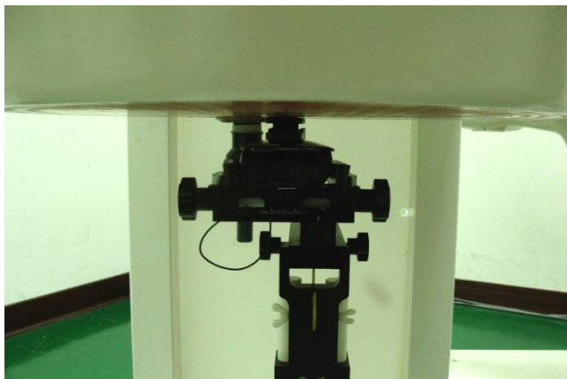
Face of the DUT with Battery 1 + Scanner 1 + Keypad 1 (Holster 1 with Phantom 0 cm Gap)
