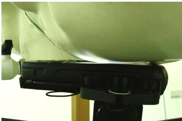
Left Cheek - DUT with Battery 1 + Scanner 1 + Keypad 1
