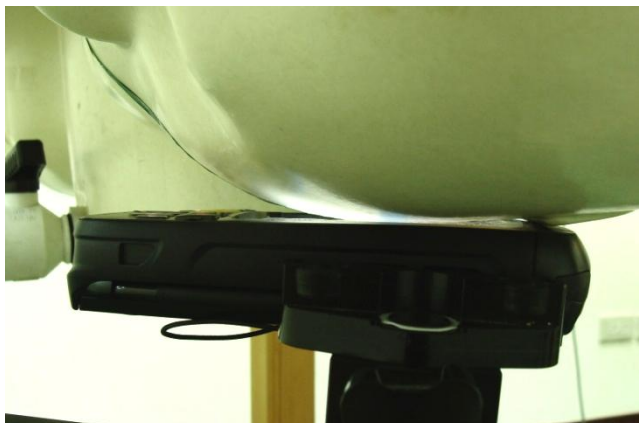
Left Cheek - DUT with Battery 1 + Scanner 2 + Keypad 1
