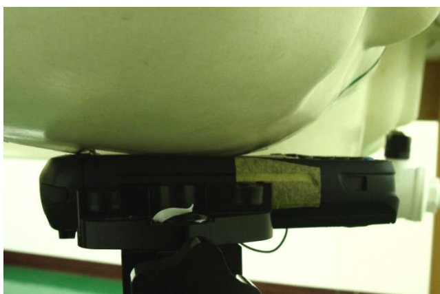
Right Cheek - DUT with Battery 1 + Scanner 1 + Keypad 2
