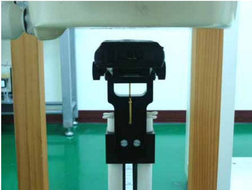
EUT Bottom with 1.5cm Gap (Sample 1)
