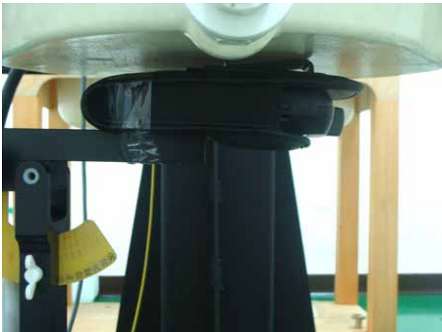
EUT Face with 0cm Gap (Sample 1 with Holster 3)
