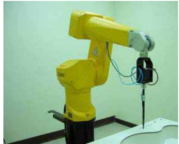
Fig. 5.2 Probe Setup on Robot
