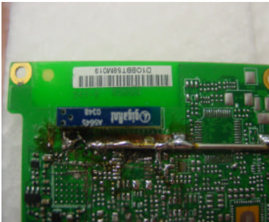
Figure 1: Mounting of the Mica antenna on the symbol scanner
