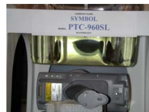
Figure 14.1 DSSS Back Body SAR Test
