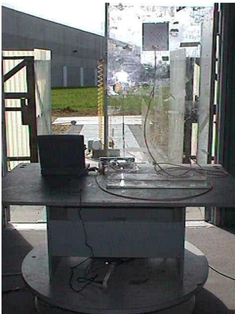
**Radiated Emission Test Setup**
