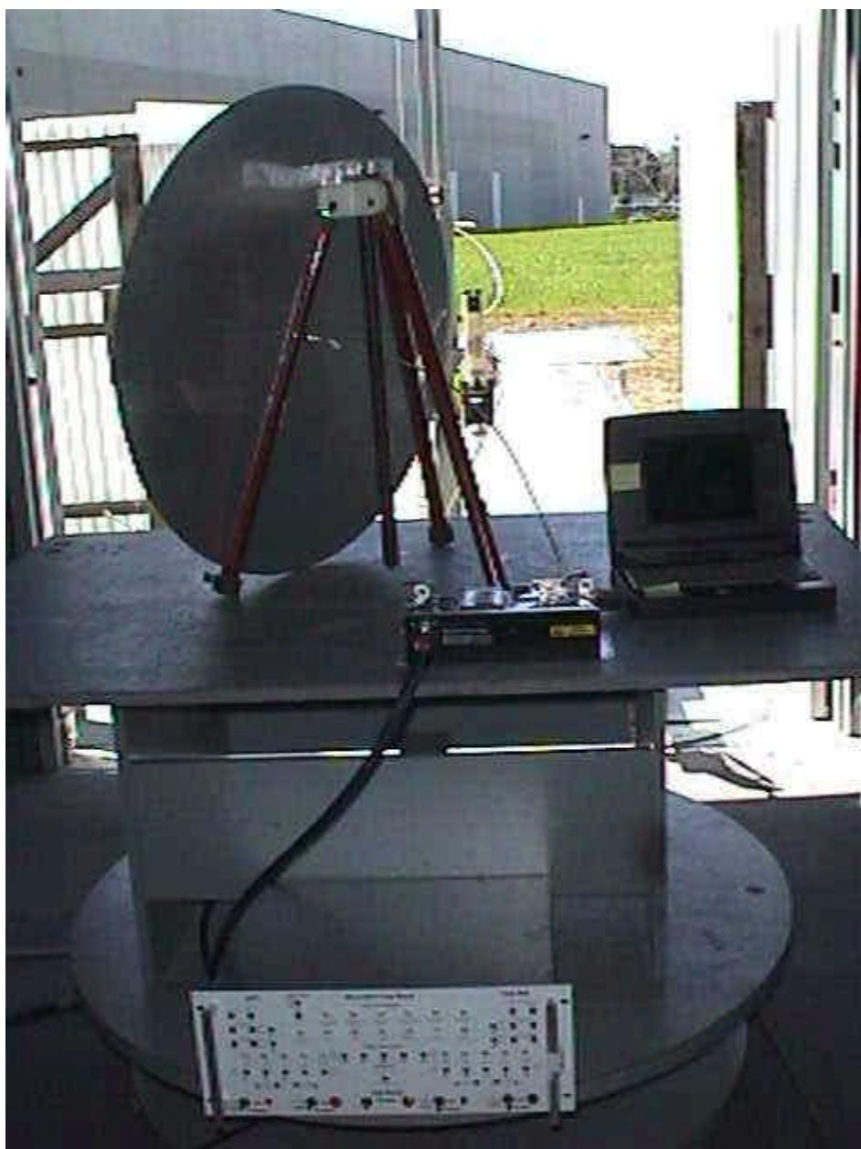
**Radiated Emission Test Setup**
