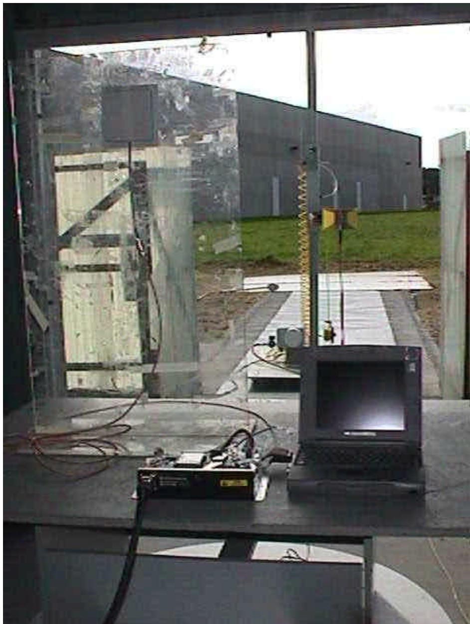
**Radiated Emission Test Setup**
